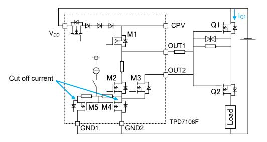
Fig. 2.7 Behavior of power reverse connection
