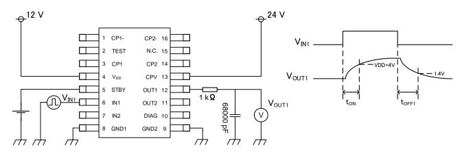
Fig. 3.1 Switching time measurement circuit 1
