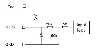
Fig. 4.1 STBY terminal equivalent circuit
