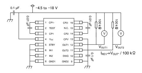
Fig. 3.4 Output current measurement circuit with power reverse connection
