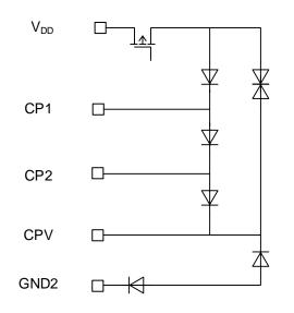
Fig. 4.3 CP1, CP2, CPV terminal equivalent circuit
