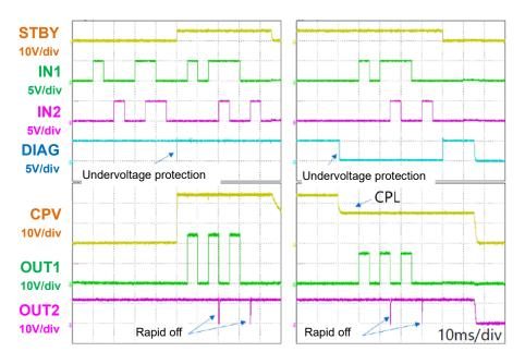
Fig. 2.6 Low voltage detection waveform
