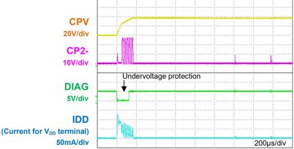
Fig. 2.4 Rising of charge pump voltage (V<sub>CPV</sub>) after releasing standby
