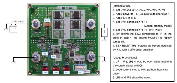
Fig. 7.3 Method of use for TPD7106F evaluation board
