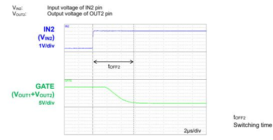
Fig. 2.3 Rapid off control waveform
