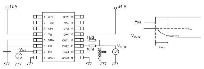
Fig. 3.3 Switching time measurement circuit 2
