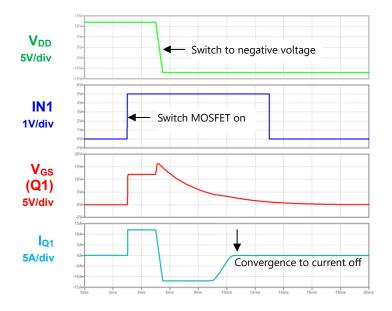
Fig. 2.8 Behavior of power reverse connection (simulation)
