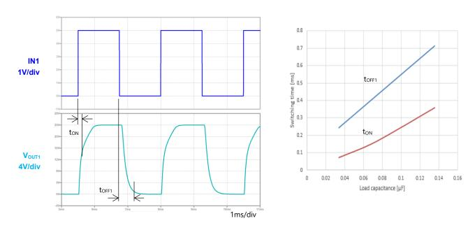
Fig. 3.2 Switching time and load capacitance (simulation)
