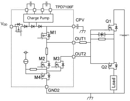
Fig. 2.1 Control of external MOSFET
