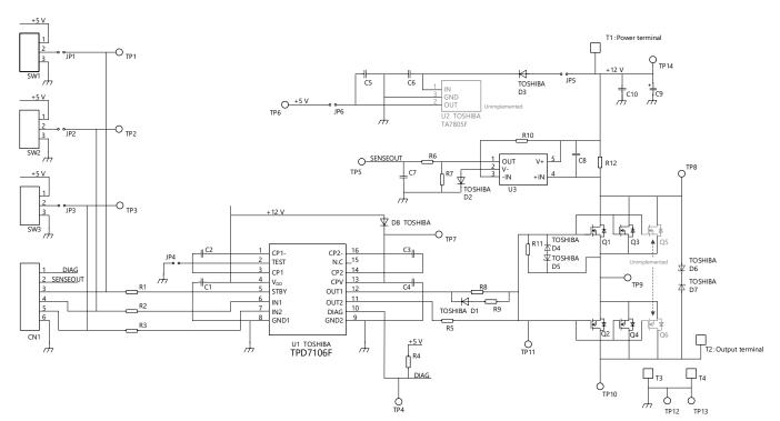
Fig. 7.4 TPD7106F evaluation board circuit diagram
