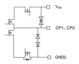
Fig. 4.4 CP1-, CP2- terminal equivalent circuit
