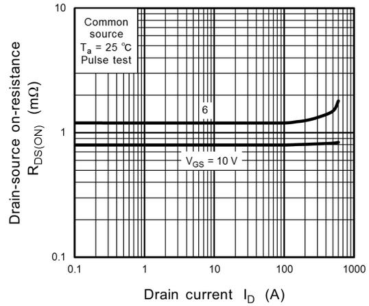
**Fig. 8.8  $R_{DS(ON)} - I_D$**
