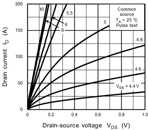
Fig. 8.1  $I_D - V_{DS}$
