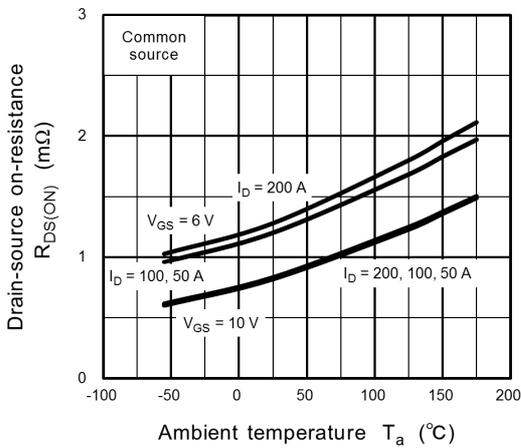
**Fig. 8.9  $R_{DS(ON)} - T_a$**
