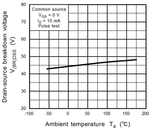
**Fig. 8.11  $V_{(BR)DSS} - T_a$**
