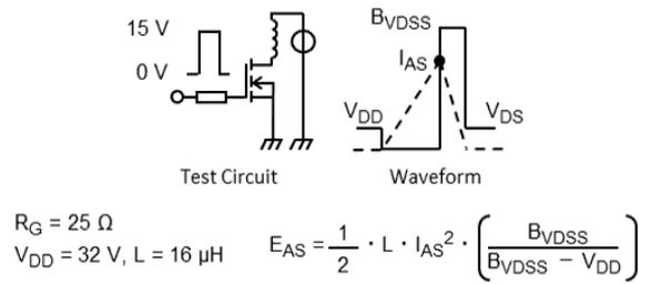
**Fig. 8.16 Test Circuit/Waveform**
