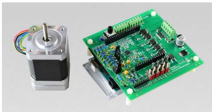
**Figure 1-1 Motor Control Closed-loop system**
