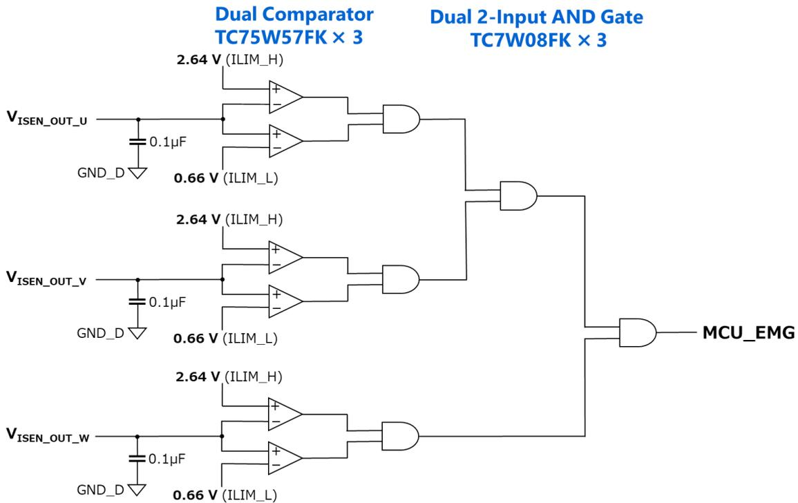
**Fig. 4.8 Overcurrent Detection Circuit**
