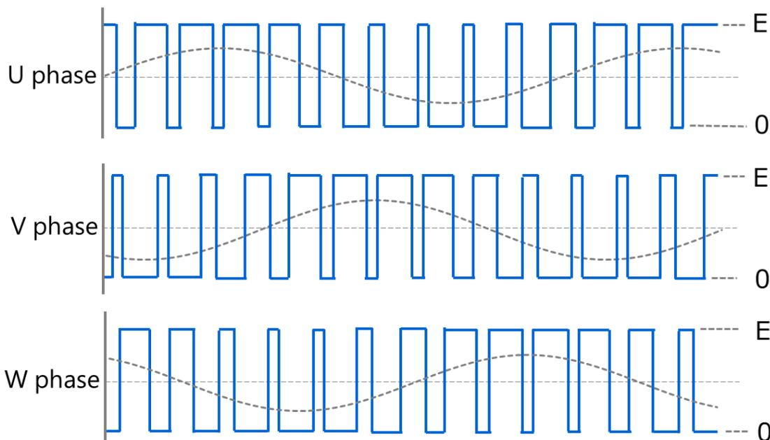
**Fig. 3.5 Example of Phase Voltage (Sine Wave) Output of 3-Phase 2-Level Inverter**
