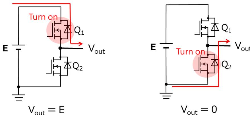
Fig. 3.2 Switching Operation of 2-Level Inverter
