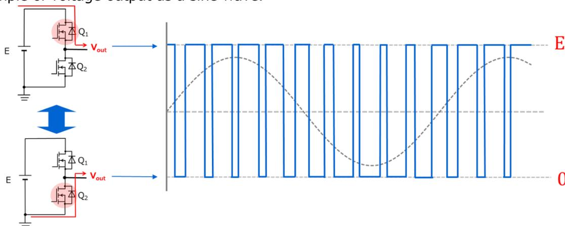
Fig. 3.3 Example of Voltage Output (Sine Wave) using a 2-Level Inverter
