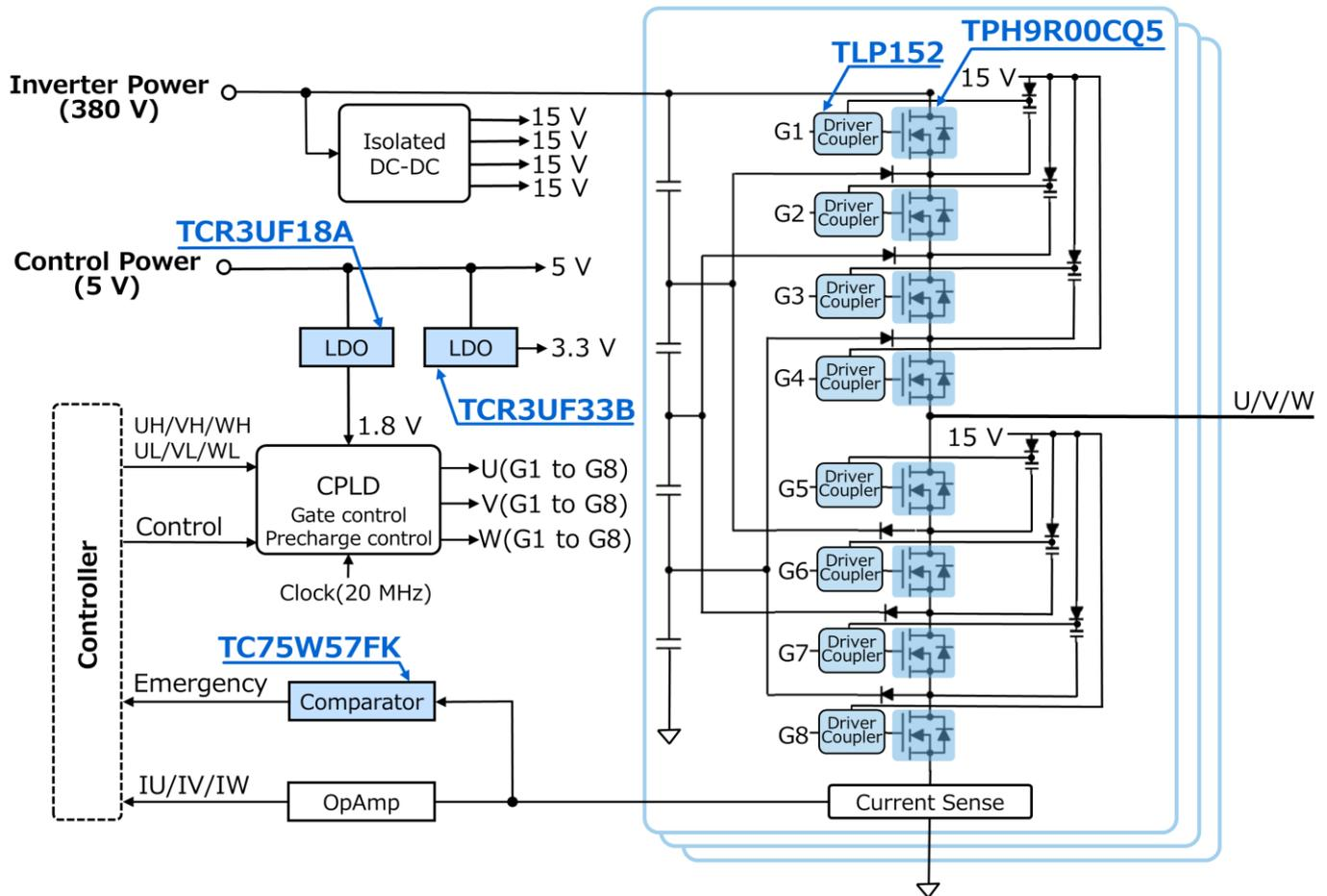
Fig. 4.1 Block Diagram of 3-Phase Multi-Level Inverter using MOSFET
