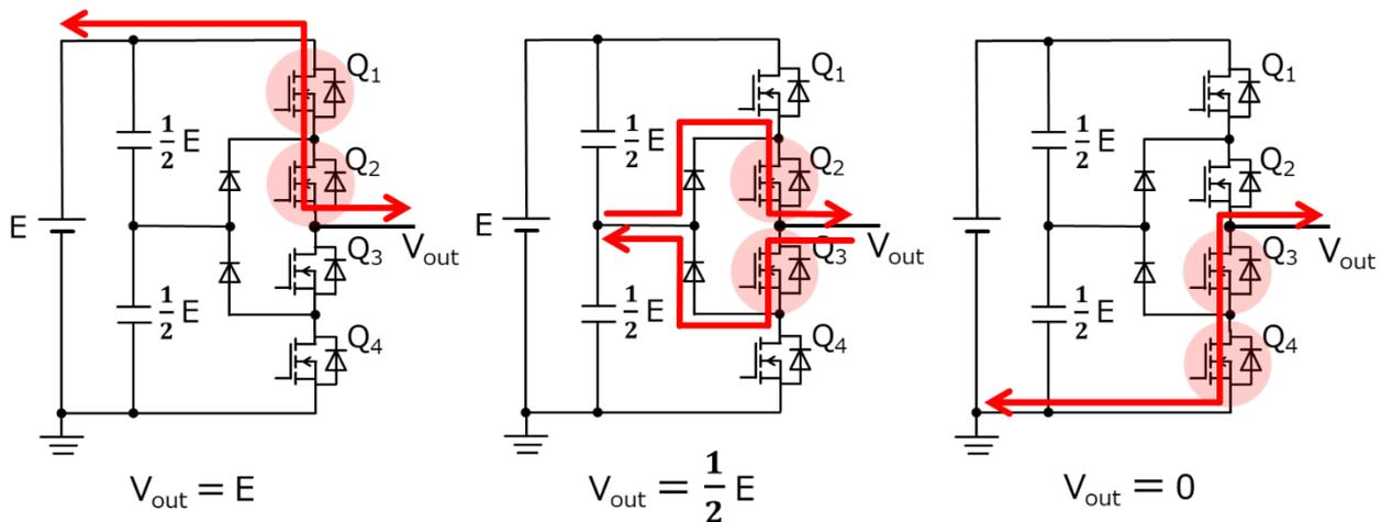
Fig. 3.6 3-Level Inverter Switching Operation
