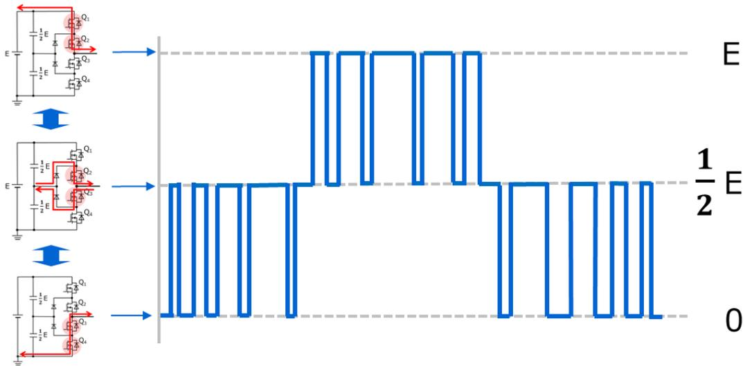
**Fig. 3.7 Example of Phase Voltage Output of 3-Level Inverter**
