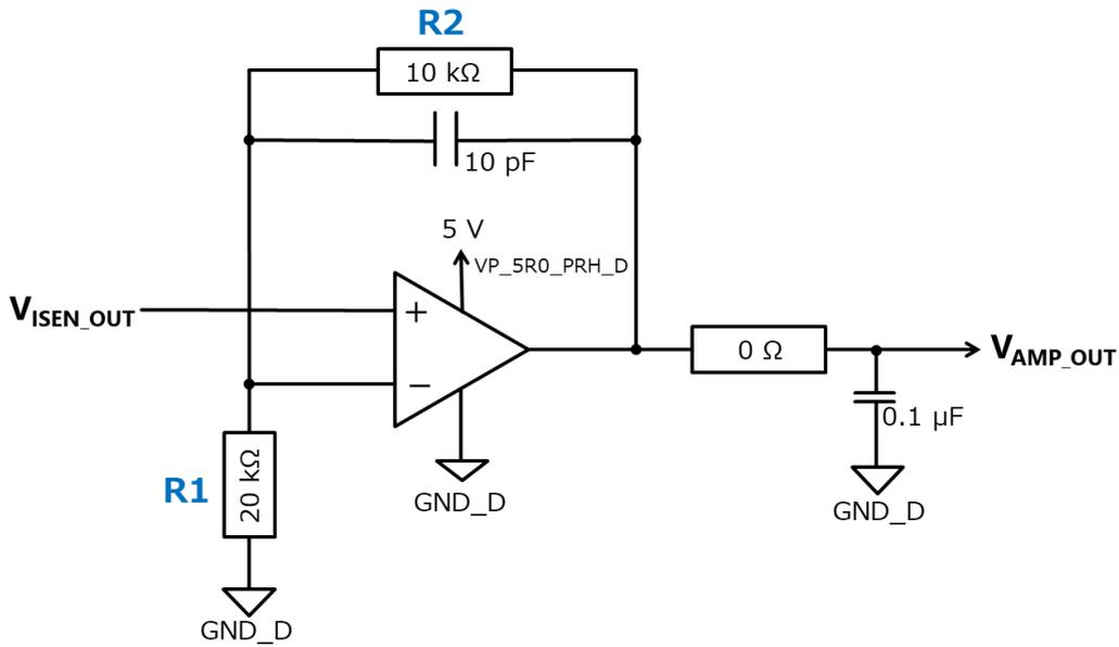
**Fig. 4.7 Current Measurement Output Circuit**
