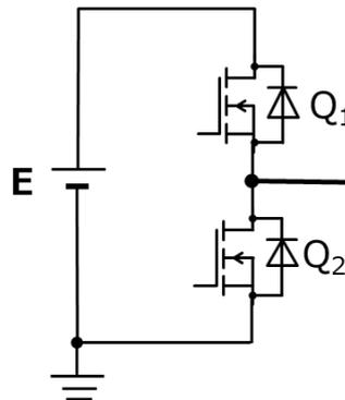
Fig. 3.1 Example of Half-Bridge Circuit
