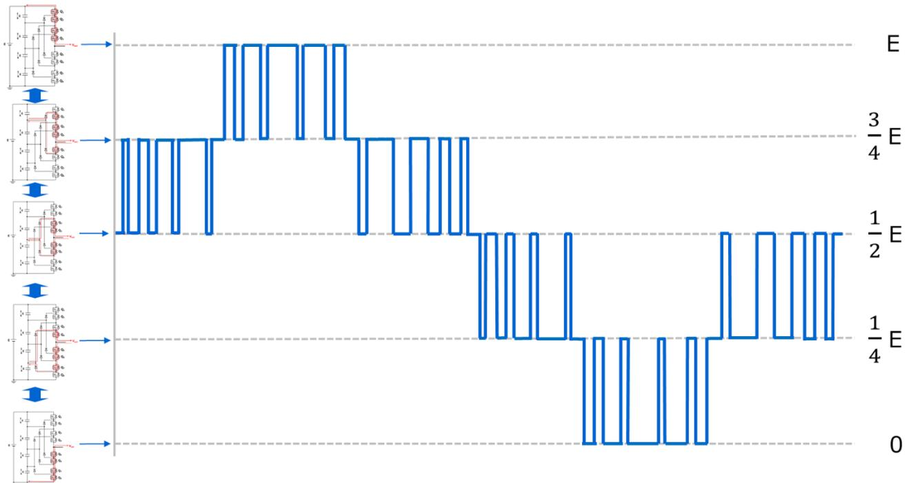
**Fig. 3.9 Example of Phase Voltage Output of 5-Level Inverter**
