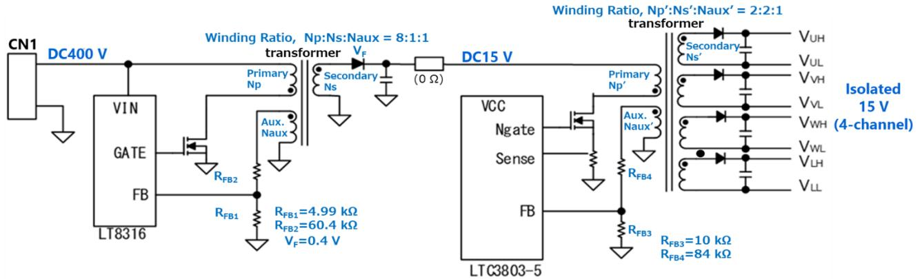
**Fig. 4.2 Isolated Power Supply Circuit**
