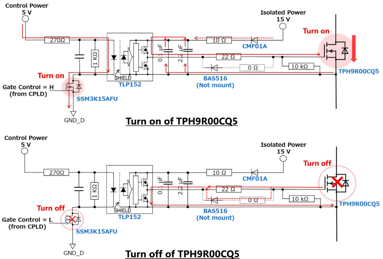
Fig. 4.5 Gate Drive Operation of MOSFET for Inverter Switching
