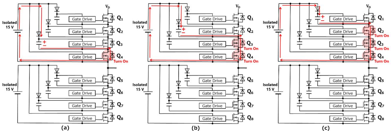
**Fig. 4.4 Charging Sequence of Gate Driver Power Supply Capacitors**
