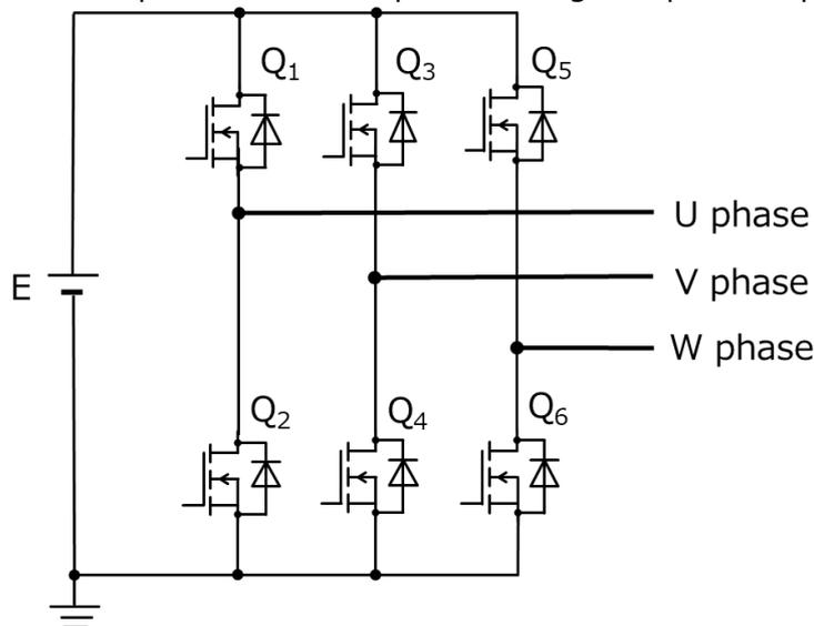
**Fig. 3.4 Configuration Example of 3-Phase 2-Level Inverter**
