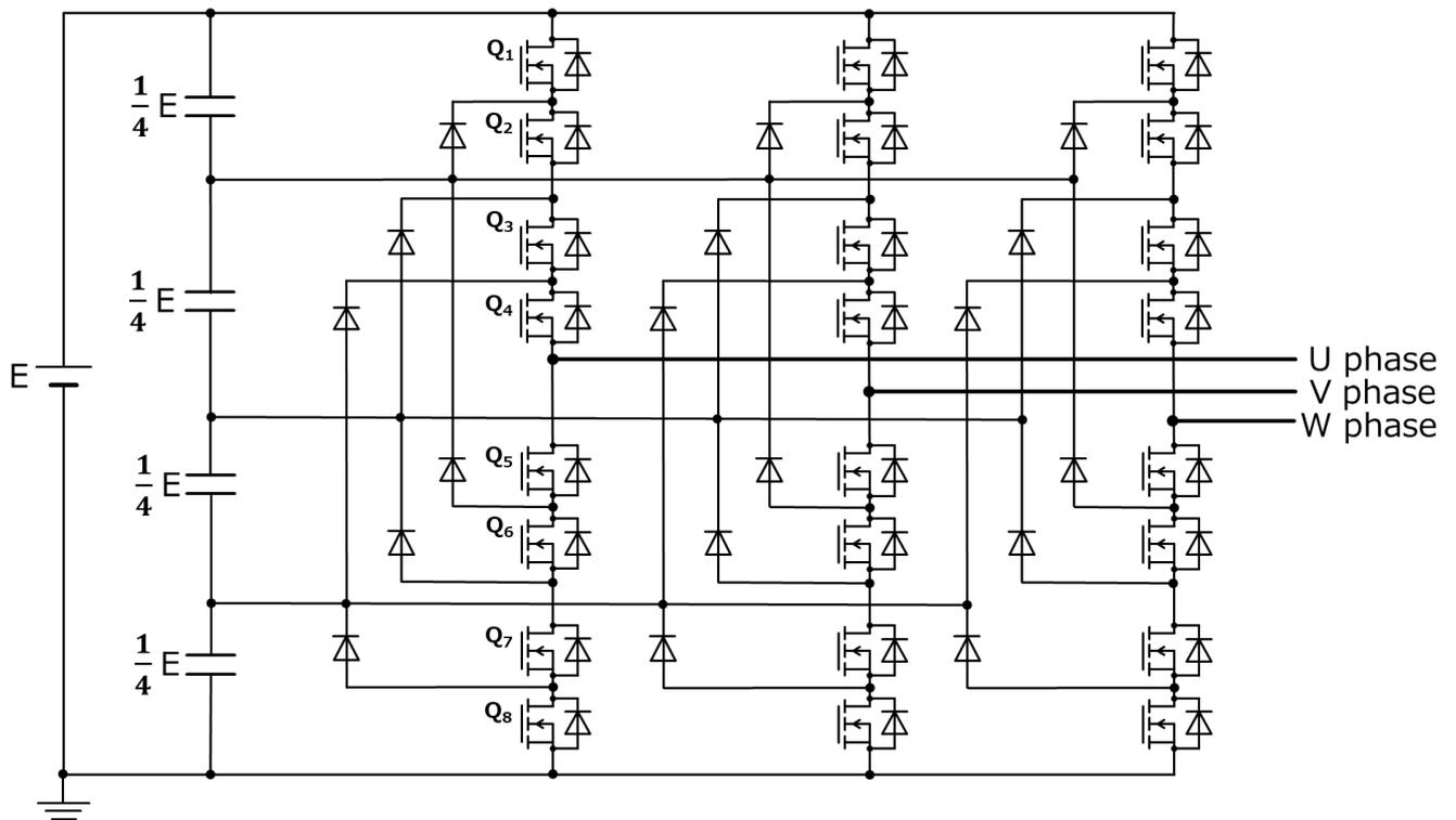
**Fig. 3.10 Example of 3-Phase, 5-Level Inverter Configuration**
