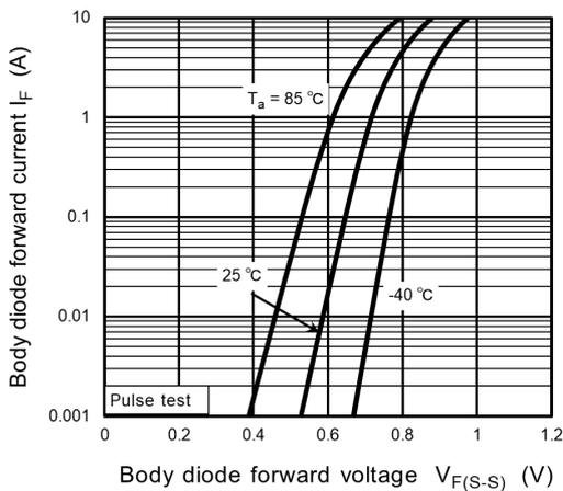
**Fig. 9.5  $I_F - V_{F(S-S)}$**
