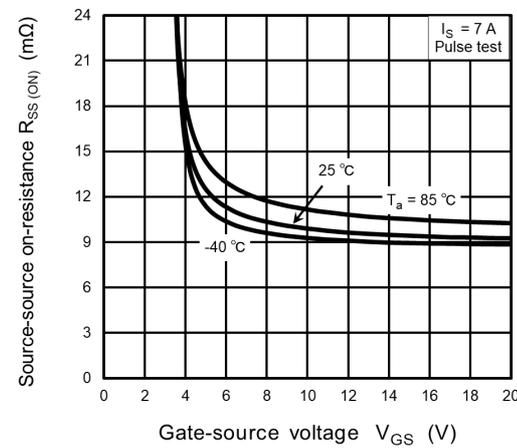
**Fig. 9.4  $R_{SS(ON)} - V_{GS}$**
