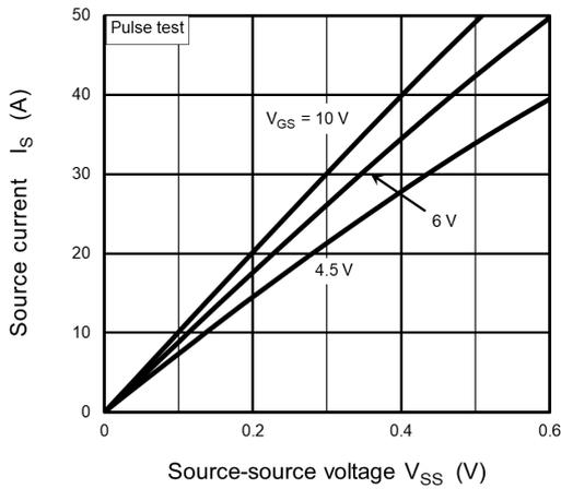
**Fig. 9.1  $I_S - V_{SS}$**
