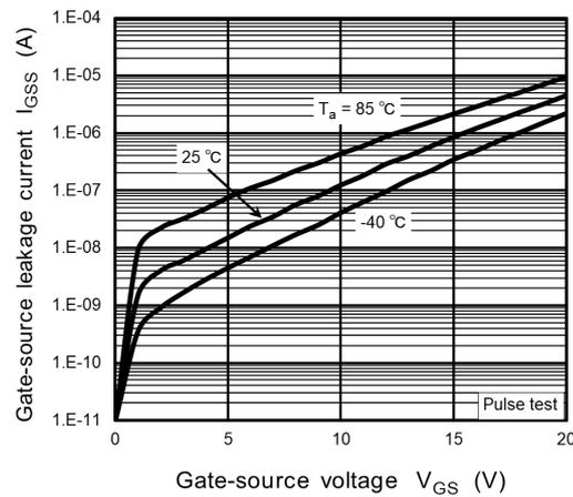
**Fig. 9.6  $I_{GSS} - V_{GS}$**
