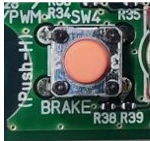
**Fig. 4.11 Brake Switch (SW4)**
