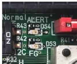
**Fig. 4.14 FG LED (DS3, Blue) and ALERT LED (DS4, Red)**
