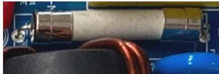
**Fig. 4.7 AC Power Supply Fuse (F1)**
