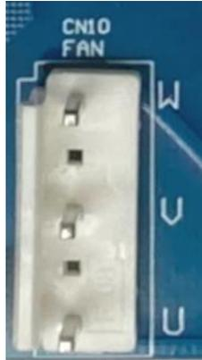
**Fig. 4.2 Fan Motor Connector (CN10)**
