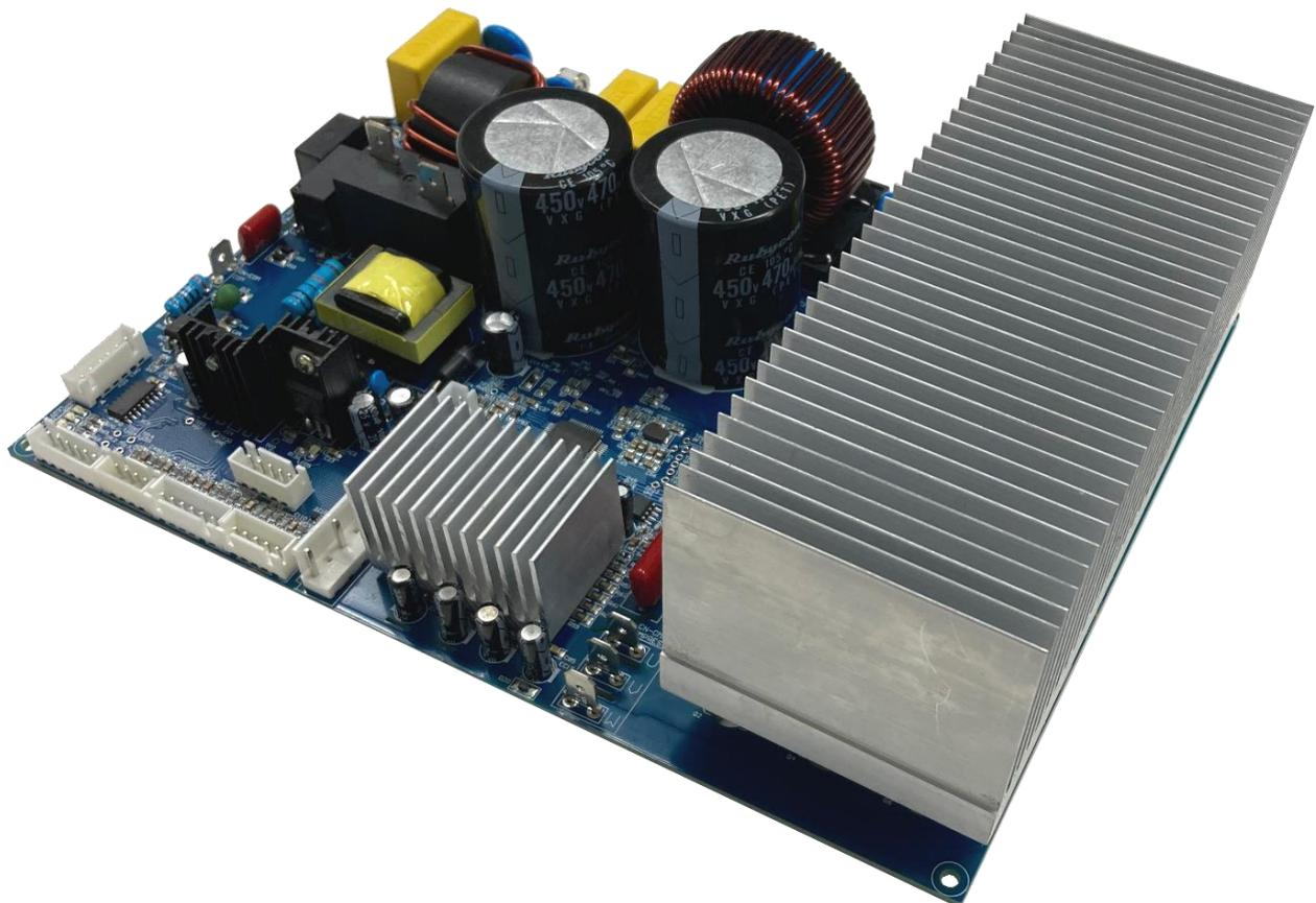
Fig. 2.4 Side View of the Air Conditioner Outdoor Unit Circuit Board
