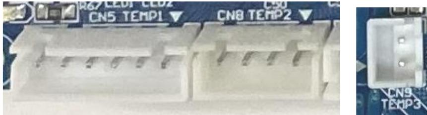
**Fig. 4.8 Temperature Sensor Connectors (CN5, CN8, CN9)**
