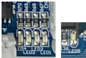
**Fig. 4.12 LEDs (LED1, LED2, LED3, LED4, LED5)**
