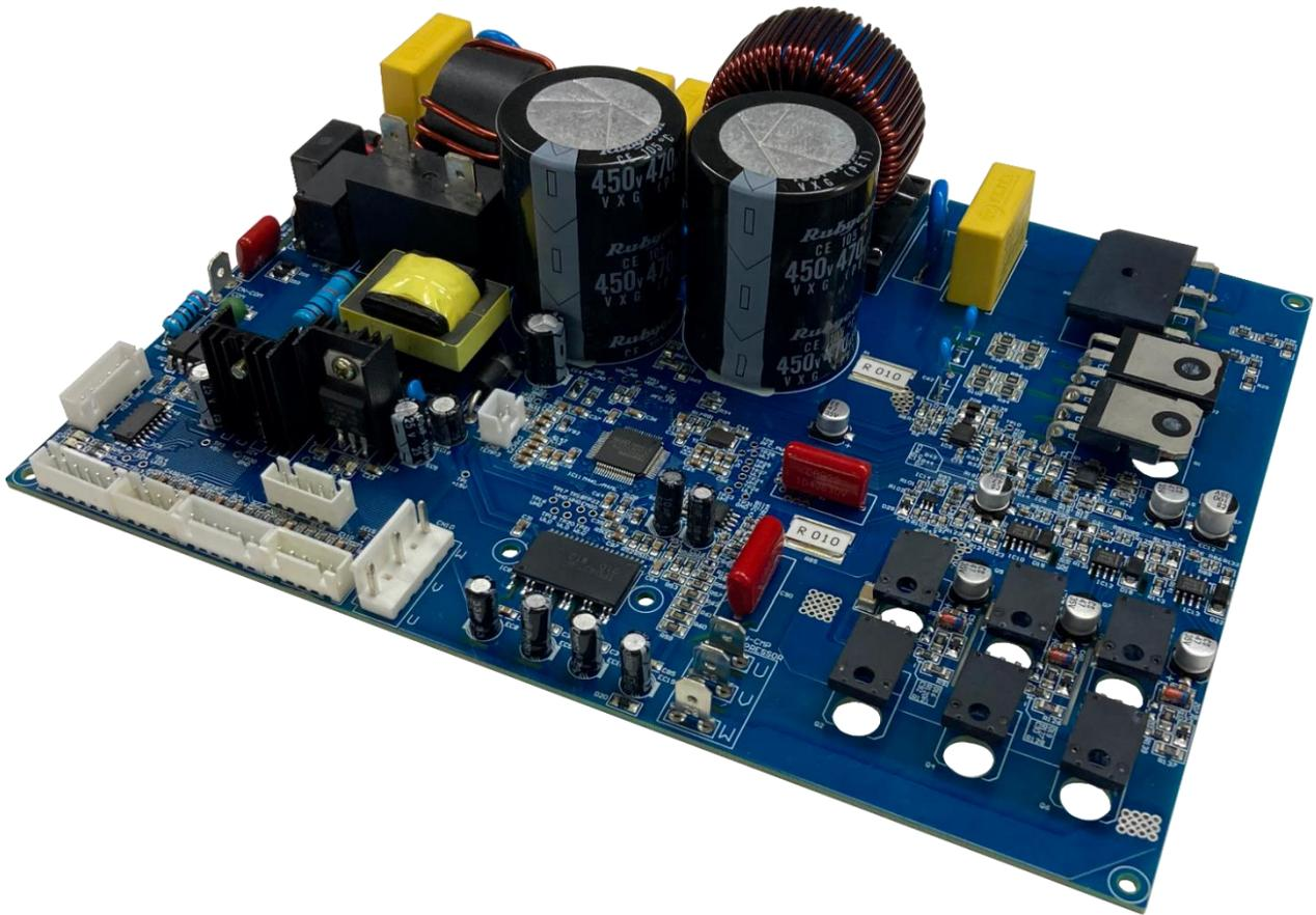
Fig. 2.3 Side View of the Air conditioner Outdoor Unit Circuit Board
