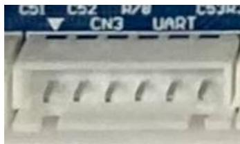
**Fig. 4.9 UART Connector (CN3)**
