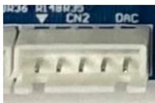
Fig. 4.11 DAC Output Connector (CN2)
