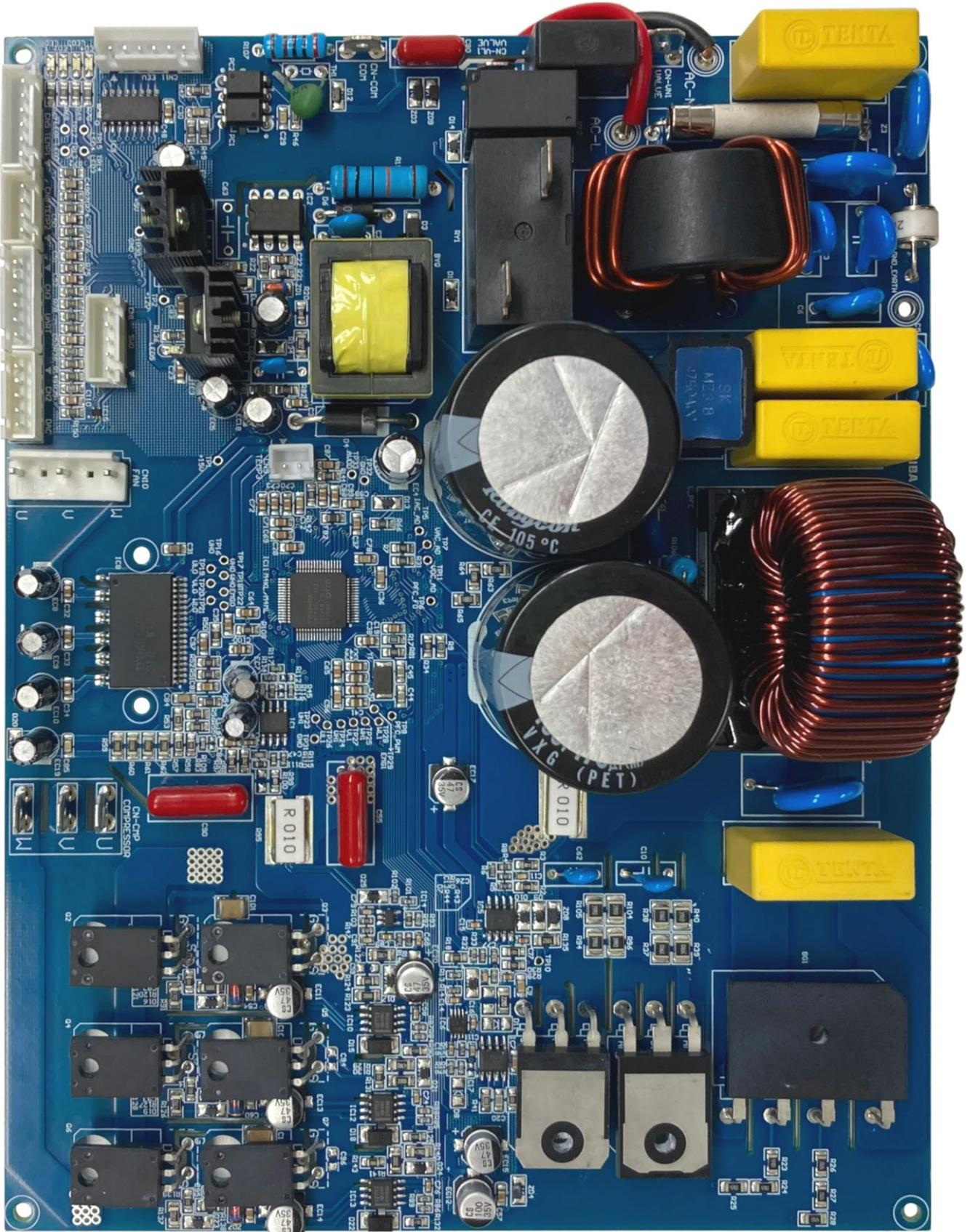
**Fig. 2.2 Front View of the Air Conditioner Outdoor Unit Circuit Board**
