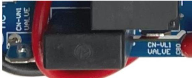
**Fig. 4.4 Four-Way Valve Connectors (CN-VL1, CN-VN1)**
