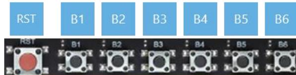
**Fig. 4.13 Host MCU Board Operation Switches (RST, B1, B2, B3, B4, B5, B6)**
