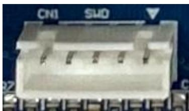
Fig. 4.10 SWD Connector (CN1)
