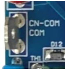
**Fig. 4.6 Indoor Unit Communication Connector (CN-COM)**
