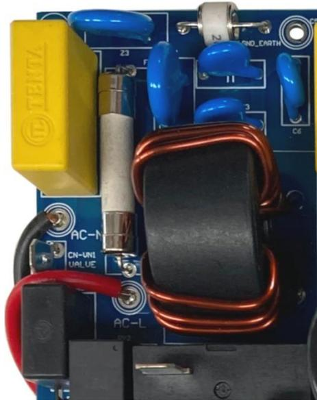
Fig. 4.1 AC Power Supply Input Terminals (AC-L, AC-N, GND\_EARTH)
