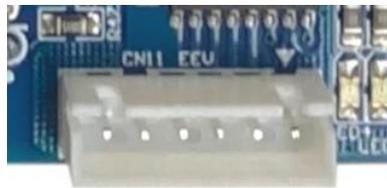
**Fig. 4.5 Electric Expansion Valve Connector (CN11)**
