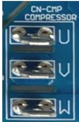
**Fig. 4.3 Compressor Connector (CN-CMP)**
