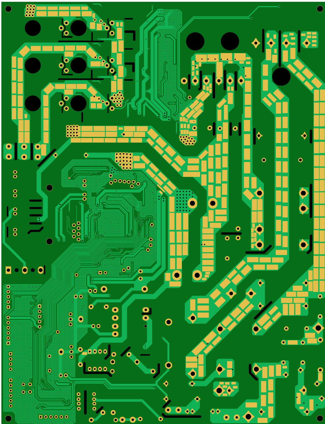
**Fig. 2.6 PCB Layout of the Main Components of the Air Conditioner Outdoor Unit Circuit (Bottom)**
