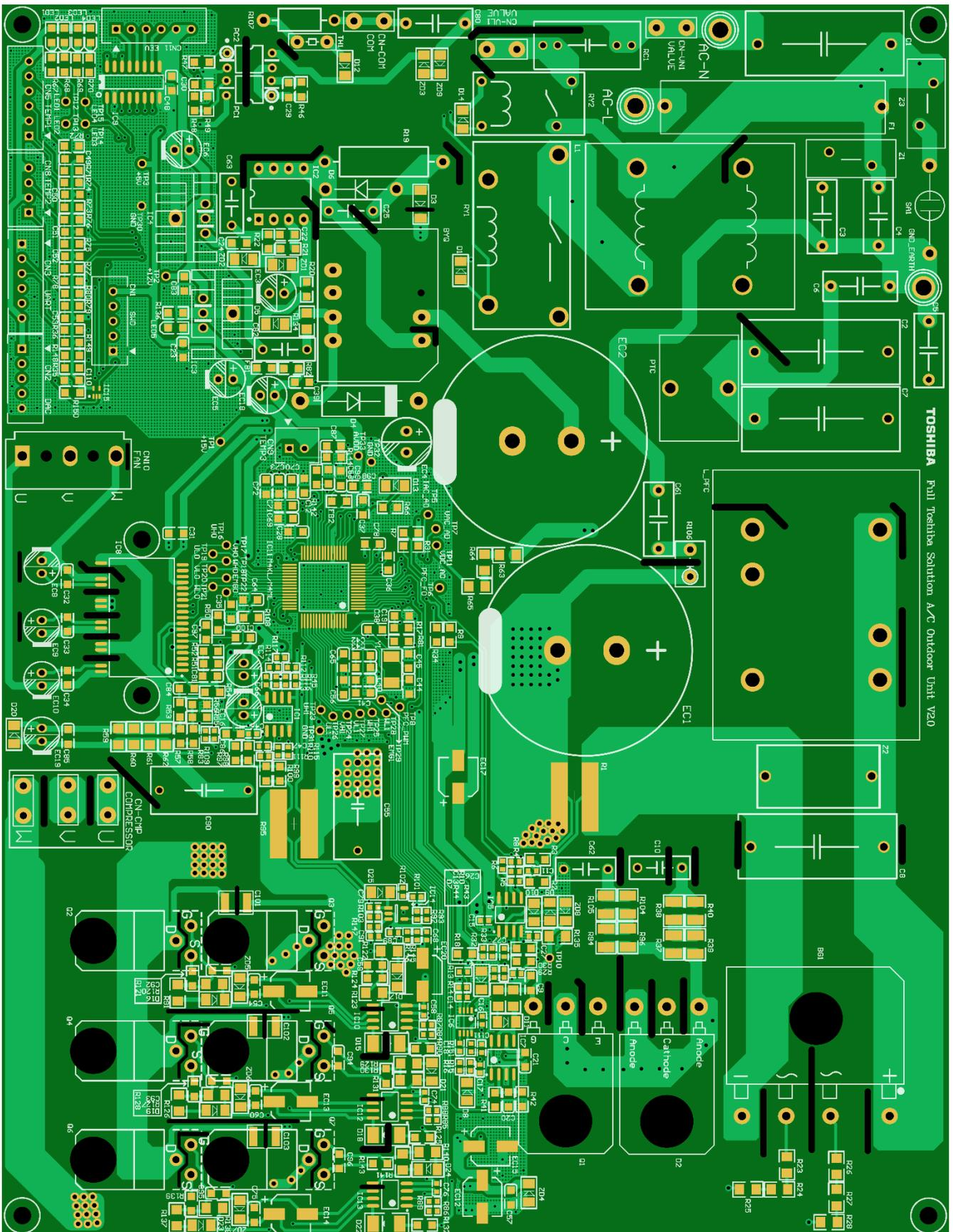
**Fig. 2.5 PCB Layout of the Main Components of the Air Conditioner Outdoor Unit Circuit (Top)**
