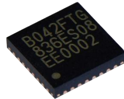
P-VQFN32-0505-0.50-005 Package (5 x 5 x 1 mm)
