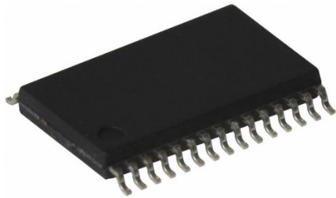
SSOP30-P-300-0.65 Package (10.2 x 7.6 x 1.6 mm)
