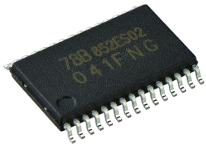
SSOP30-P-300-0.65 Package (10.2 x 7.6 x 1.6 mm)
