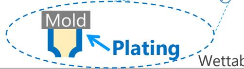
Wettable Flank (WF) structure
