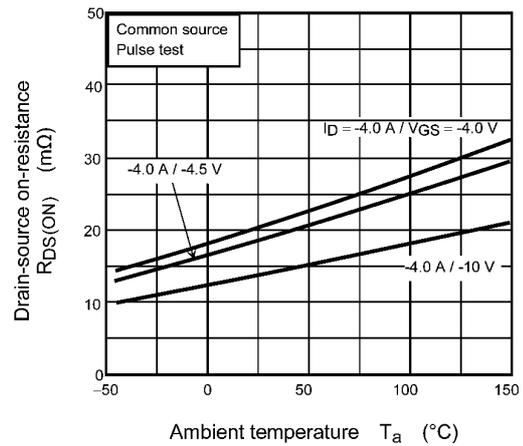
Fig. 8.6  $R_{DS(ON)} - T_a$
