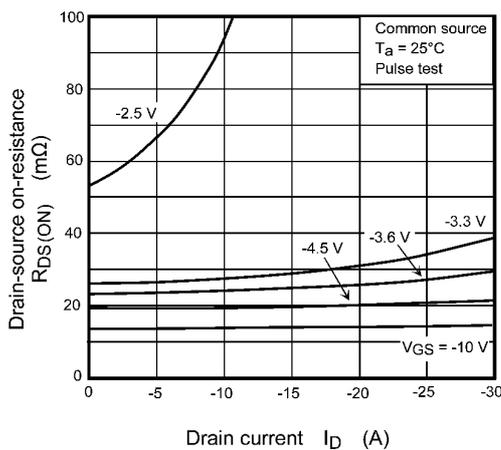
Fig. 8.5  $R_{DS(ON)} - I_D$
