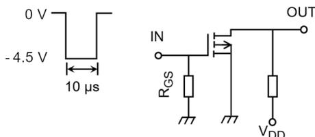
Fig. 5.3.1 Switching Time Test Circuit
