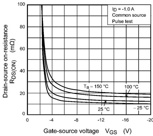
Fig. 8.3  $R_{DS(ON)} - V_{GS}$
