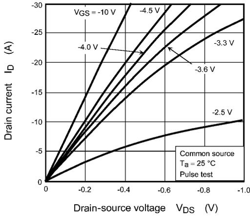
Fig. 8.1  $I_D - V_{DS}$
