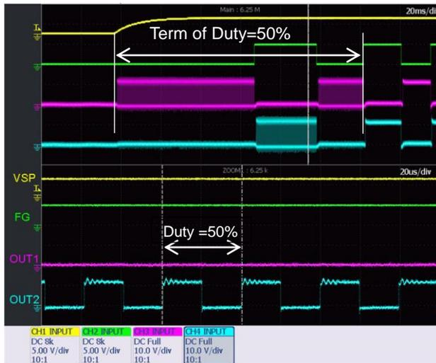
Figure 3.3 Operation waveform in output start (Output in startup Duty=50%)
