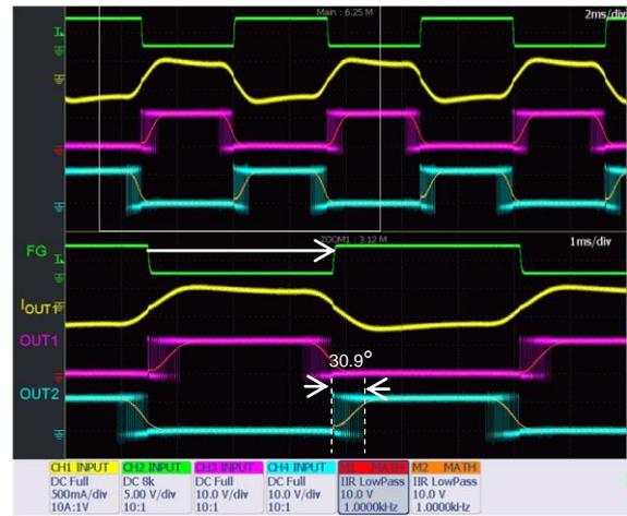
Figure 3.6 Operation waveform of the IC (Soft switching term: 30.9°)
