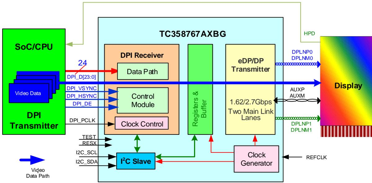
**Figure 1.2 System Overview with TC358767AXBG in MODE\_P21 Configuration**
