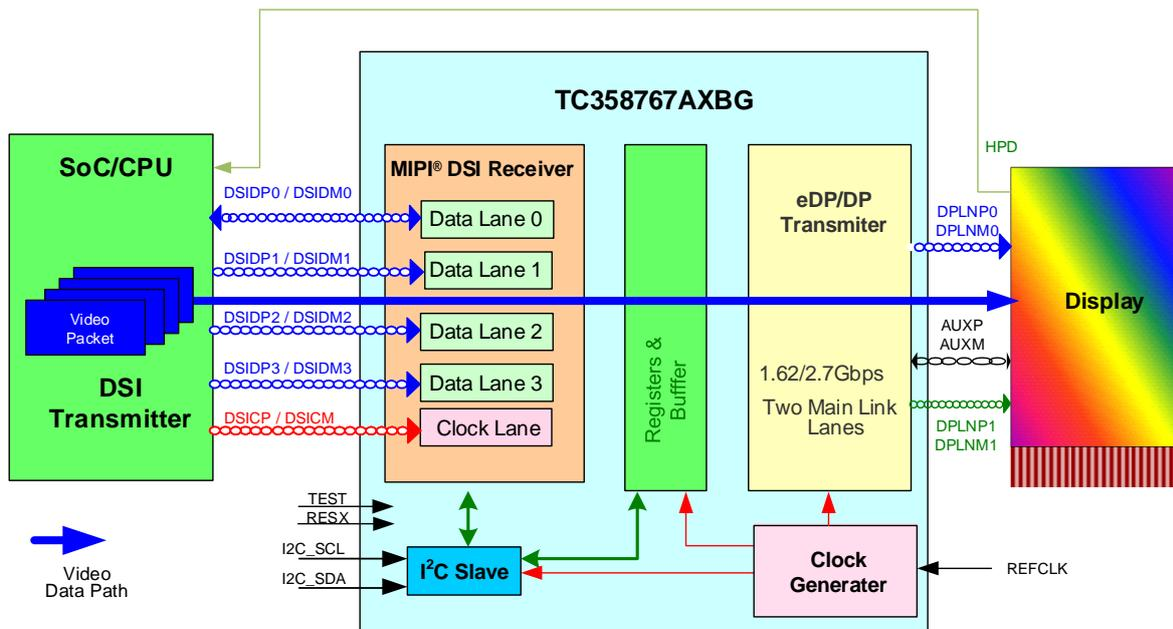
**Figure 1.1 System Overview with TC358767AXBG in MODE\_S21 Configuration**
