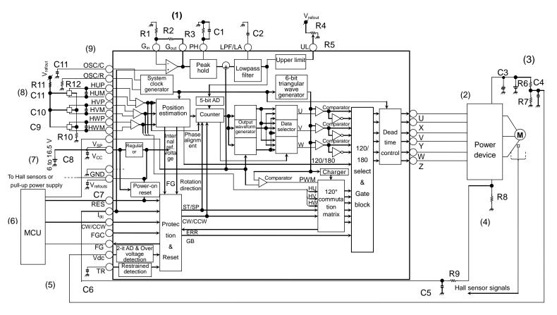
Figure 1 Application circuit example
