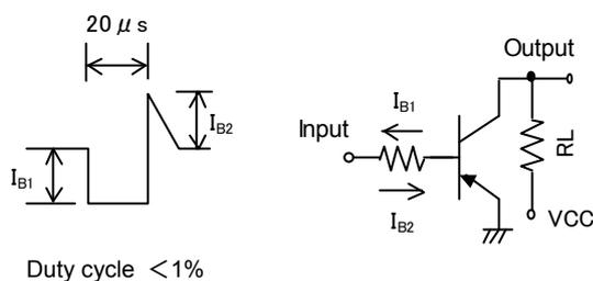
Figure 4. Switching Time Test Circuit & Timing Chart
