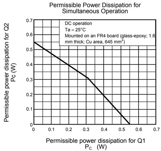
Collector power dissipation at single-device operation is 0.55 W.
