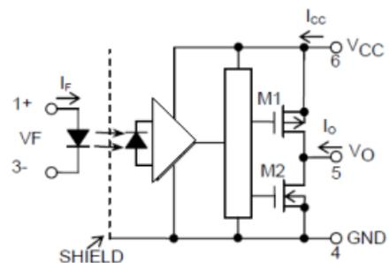
A ceramic capacitor (0.1 μF) should be connected from pin 6 (VCC) to pin 4 (GND) to stabilize the operation of the high gain linear amplifier. Failure to provide the bypass may impair the switching property. The total lead length between capacitor and coupler should not exceed 1 cm.
