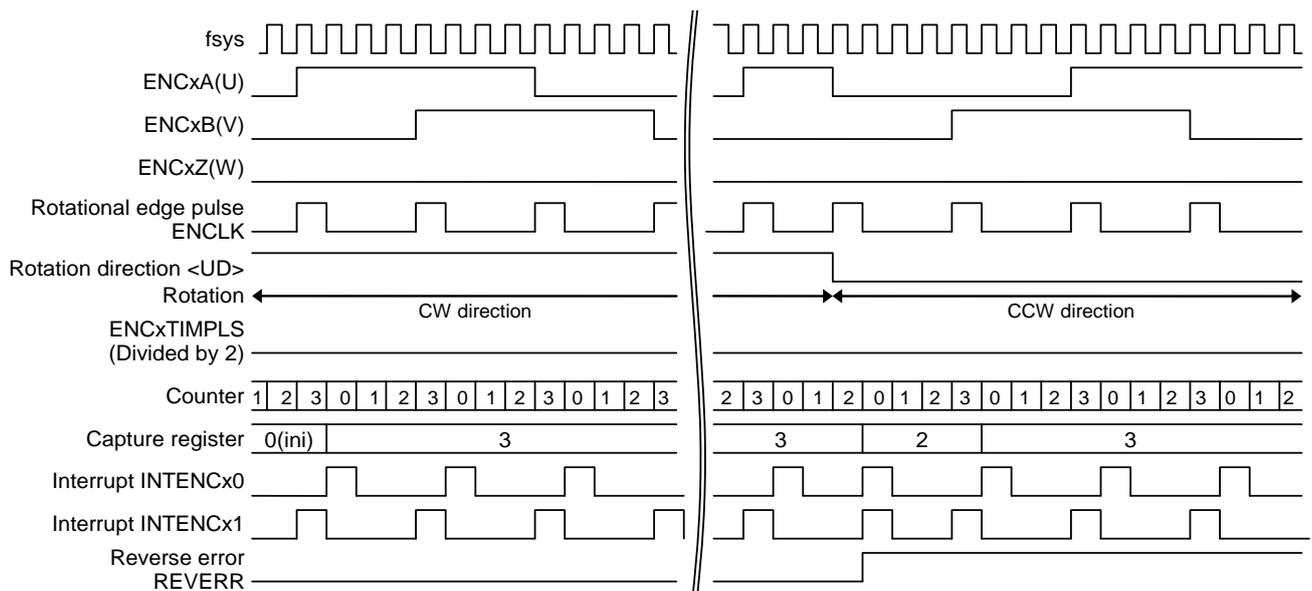
Figure 3.6 2-phase decoding ( $[ENxTNCr] <P3EN> = 0$ )
