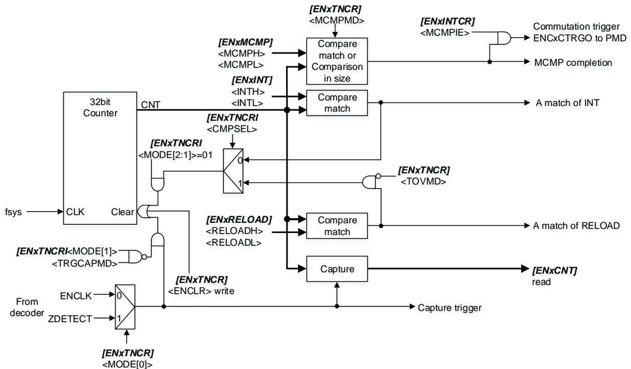
**Figure 3.23 Configuration of the counter (sensor mode (timer count) or timer mode)**
