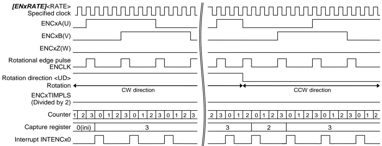
Figure 3.8 2-phase decoding ( $[ENxTNCr] <P3EN>=0$ )
