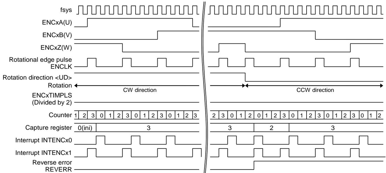
Figure 3.5 3-phase decoding ( $[ENxTNCr] <P3EN> = 1$ )
