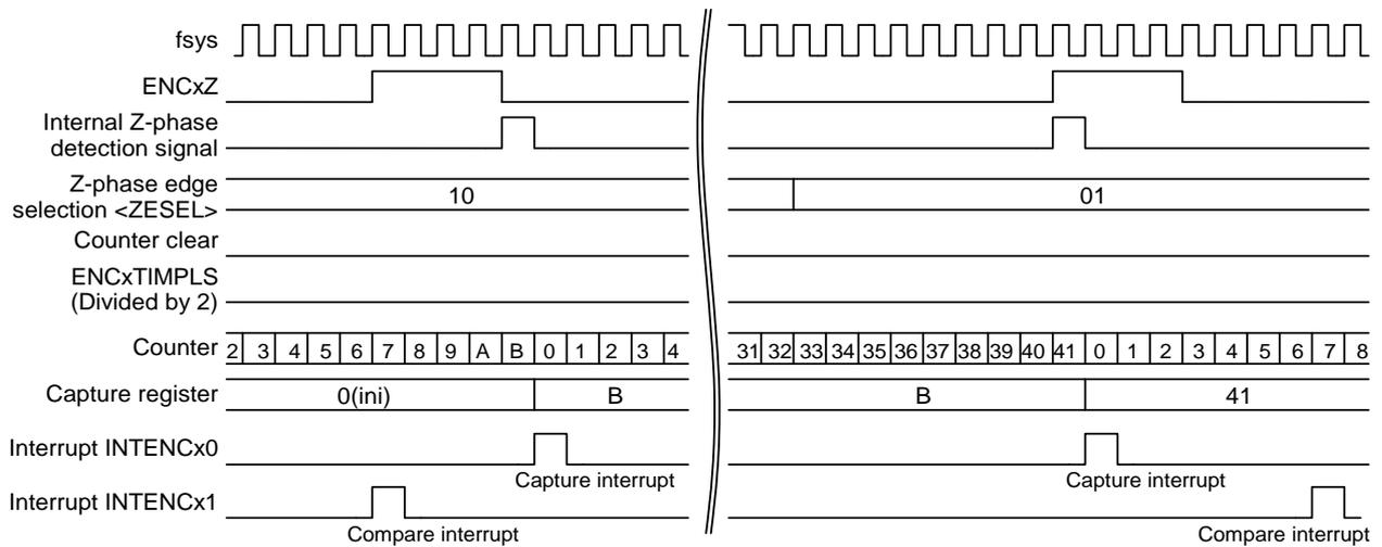
**Figure 3.9 ENCxZ input is enabled. ( $[ENxTNCr]<ZEN>=1$ )**
