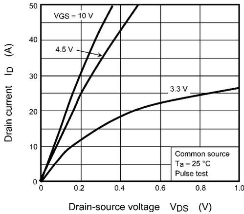
**Fig. 7.1**  $I_D - V_{DS}$
