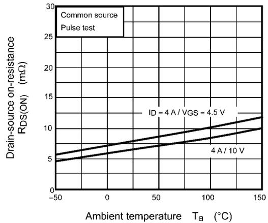
**Fig. 7.6**  $R_{DS(ON)} - T_a$
