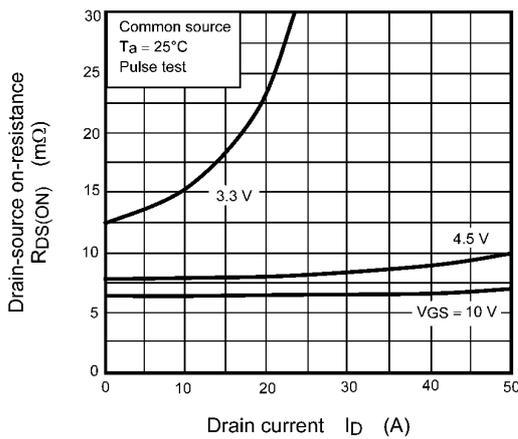
**Fig. 7.5**  $R_{DS(ON)} - I_D$
