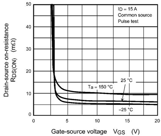
**Fig. 7.4**  $R_{DS(ON)} - V_{GS}$
