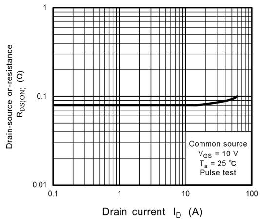
**Fig. 8.6**  $R_{DS(ON)} - I_D$
