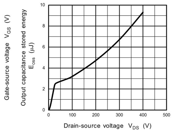
**Fig. 8.12  $E_{oss} - V_{DS}$**
