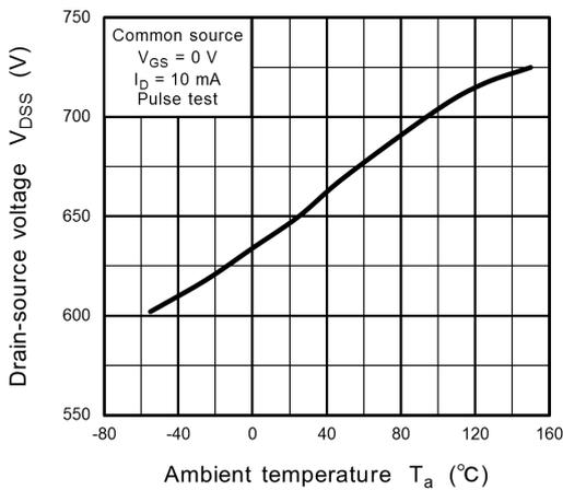
**Fig. 8.5**  $V_{DS} - T_a$
