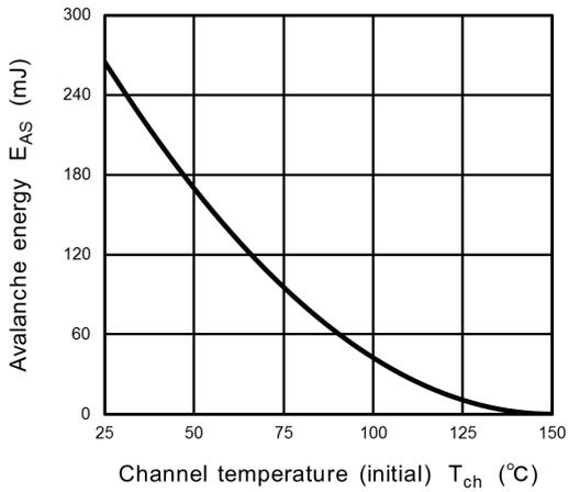
**Fig. 8.14  $E_{AS} - T_{ch}$**
