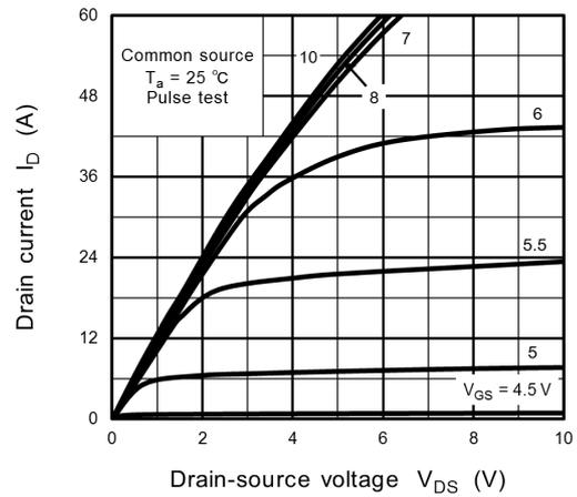
**Fig. 8.2**  $I_D - V_{DS}$
