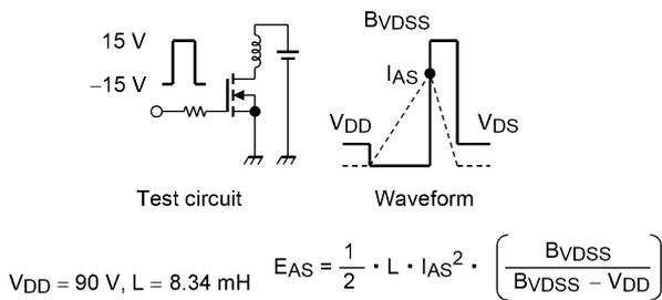
**Fig. 8.16 Test Circuit/Waveform**
