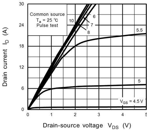
**Fig. 8.1**  $I_D - V_{DS}$
