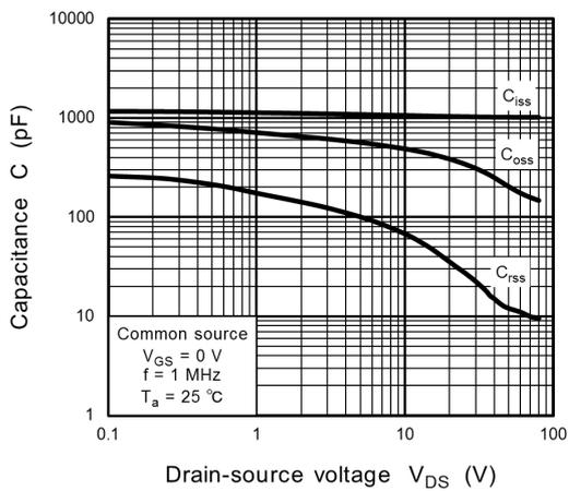
**Fig. 8.11** Capacitance -  $V_{DS}$
