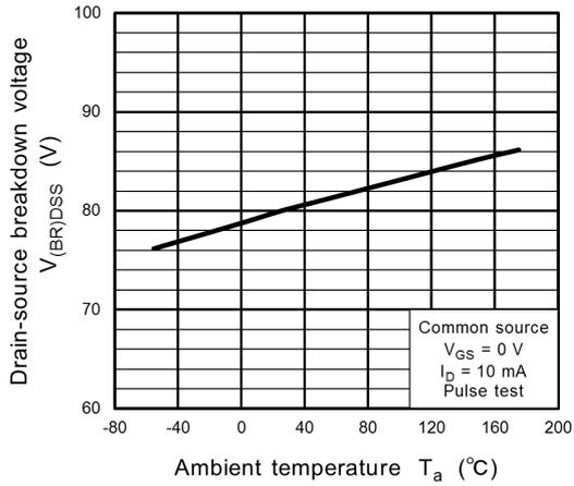
**Fig. 8.7**  $V_{(BR)DSS} - T_a$
