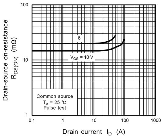
Fig. 8.5  $R_{DS(ON)} - I_D$
