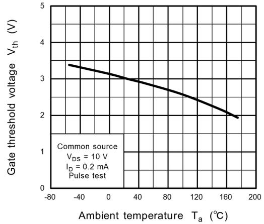
**Fig. 8.8**  $V_{th} - T_a$
