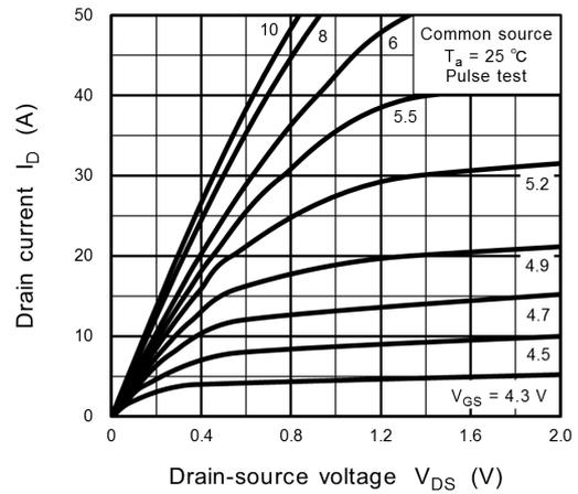
Fig. 8.2  $I_D - V_{DS}$
