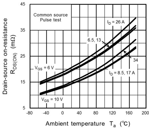
**Fig. 8.9**  $R_{DS(ON)} - T_a$
