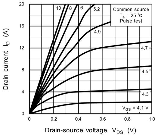
Fig. 8.1  $I_D - V_{DS}$
