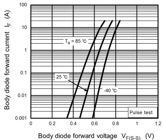
**Fig. 9.4  $I_F - V_{F(S-S)}$**
