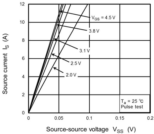
**Fig. 9.1  $I_S - V_{SS}$**
