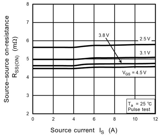
**Fig. 9.2  $R_{SS(ON)} - I_S$**
