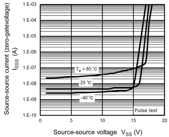
**Fig. 9.6  $I_{SS} - V_{SS}$**
