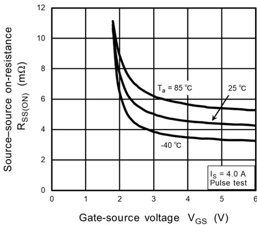
**Fig. 9.3  $R_{SS(ON)} - V_{GS}$**
