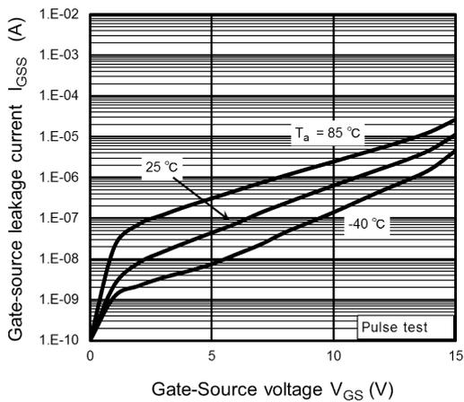
**Fig. 9.5  $I_{GSS} - V_{GS}$**
