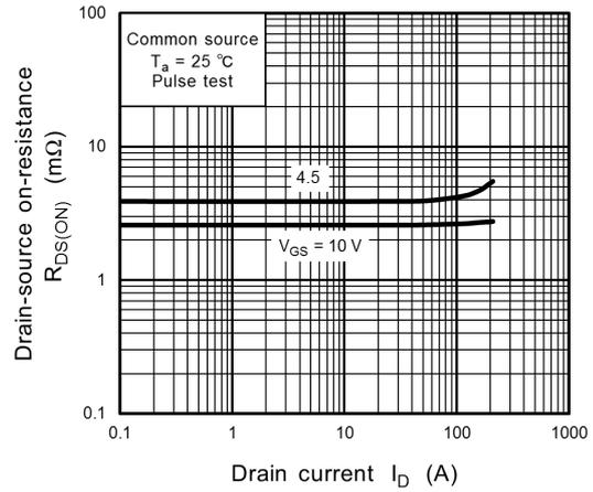
**Fig. 8.8  $R_{DS(ON)} - I_D$**
