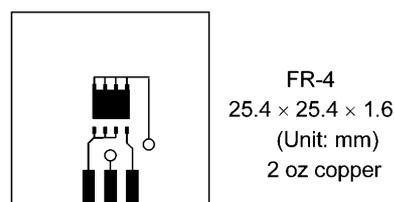
Fig. 5.2 Device Mounted on a Glass-Epoxy Board (b)
