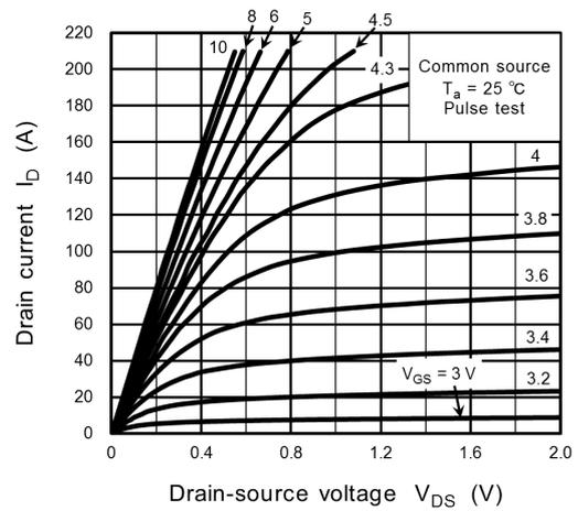
**Fig. 8.2  $I_D - V_{DS}$**
