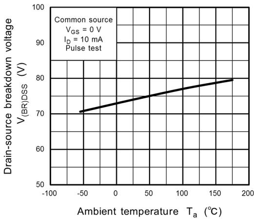
**Fig. 8.11  $V_{(BR)DSS} - T_a$**
