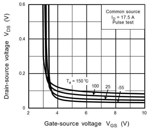
**Fig. 8.4  $V_{DS} - V_{GS}$**
