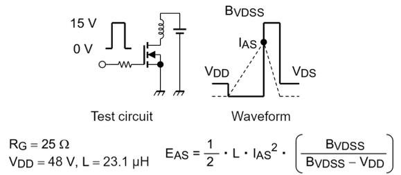
**Fig. 8.16 Test Circuit/Waveform**
