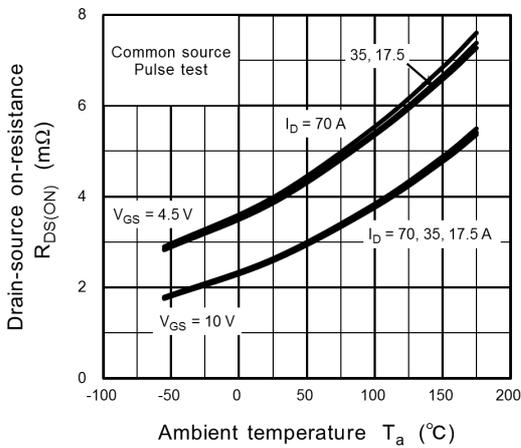
**Fig. 8.9  $R_{DS(ON)} - T_a$**
