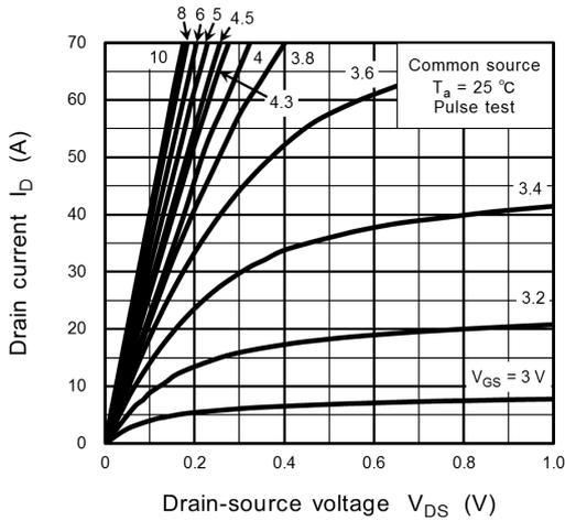
**Fig. 8.1  $I_D - V_{DS}$**
