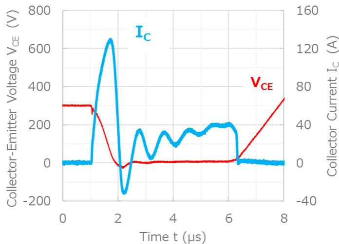
**Figure. 3-12 Example of waveform at power on (actual measurement)**
