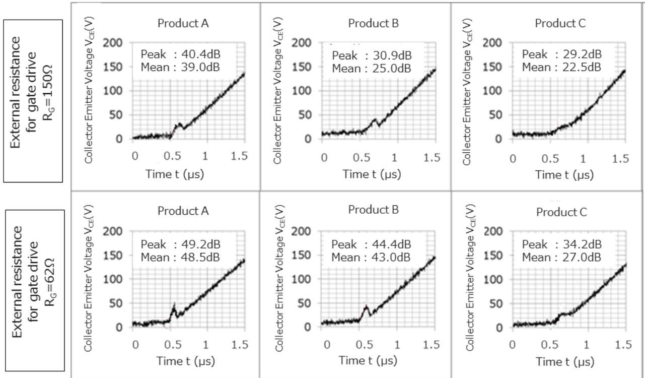
**Figure. 3-6 “ $\Delta V_{CE}$ ” waveforms and radiated emission (actual measurement)**
