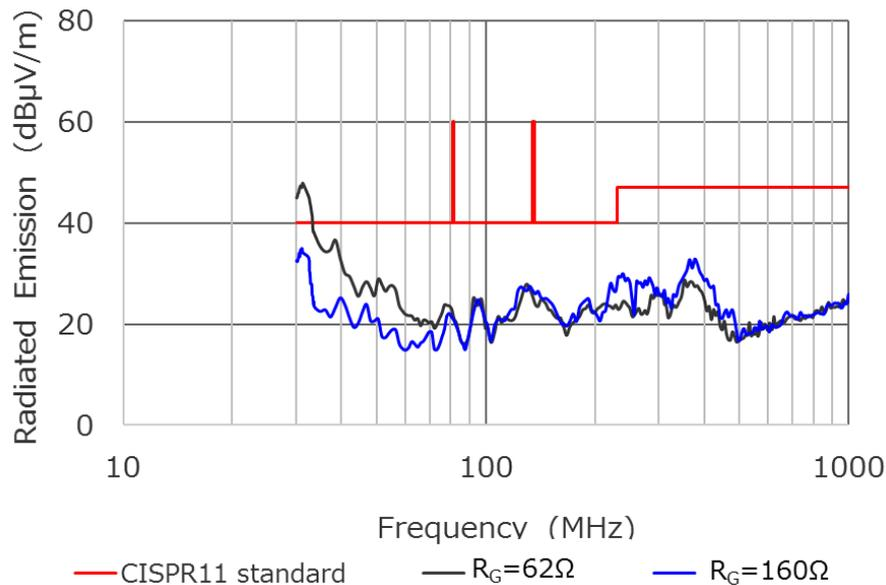
**Figure. 3-1 Radiated emission by Changing  $R_G$  in IH Rice Cooker (Actual Measurement)**
