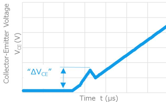
**Figure. 3-5 Defining  $V_{CE}$  Waveforms Related to radiated emission**
