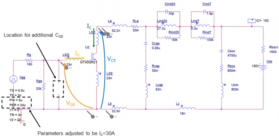
**Figure. 3-7 Model of Voltage Resonance Circuit for IH Rice Cooker (Simulation)**
