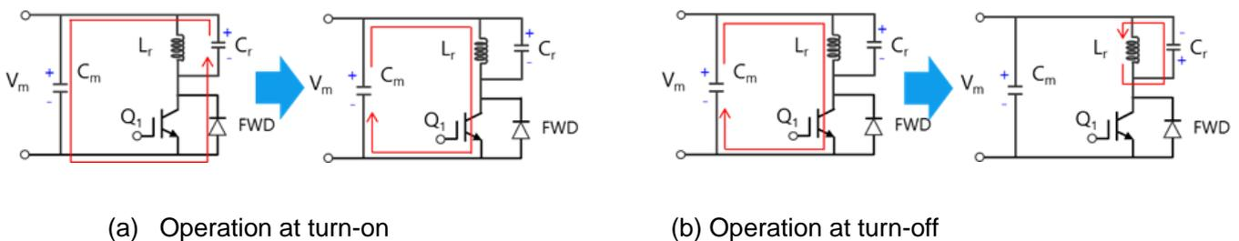
Figure. 2-3 Operation of IGBT in Voltage Resonant Circuit
