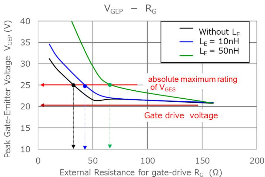
(b)  $V_{GEP}$  depends on  $R_G$  and  $L_E$
