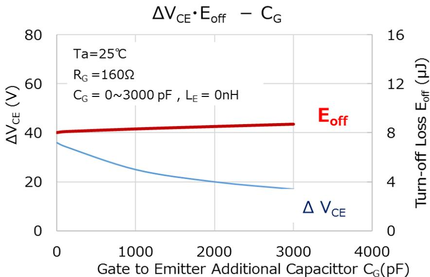
**Figure. 3-10  $C_G$  Effects on Turnoff Loss and “ $\Delta V_{CE}$ ” (Simulation)**
