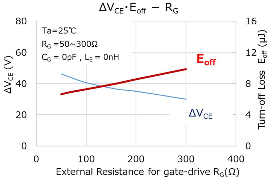
**Figure. 3-9  $R_G$  Effects on Turnoff Loss and “ $\Delta V_{CE}$ ” (Simulation)**
