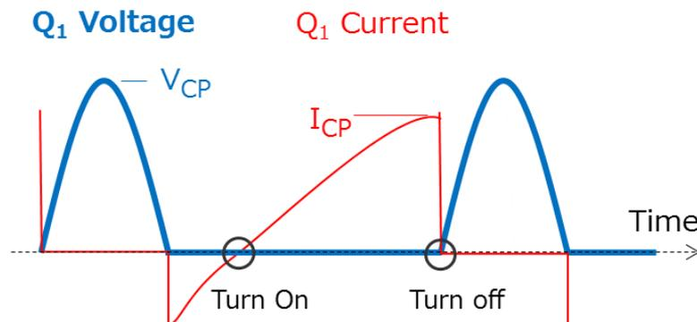
Figure. 2-2 Current and Voltage Waveforms of IGBT in Voltage Resonant Circuit
