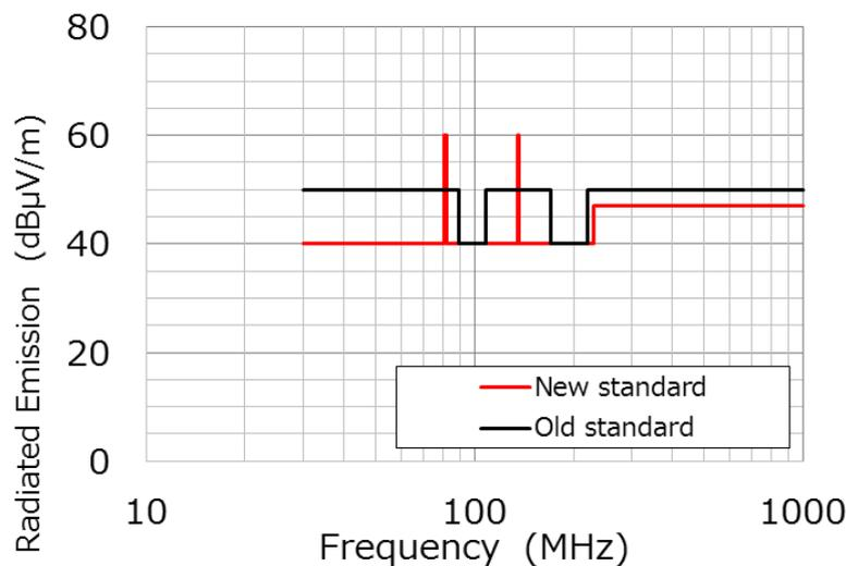
**Figure. 1-2 Old and New Radiation Noise Standard**
