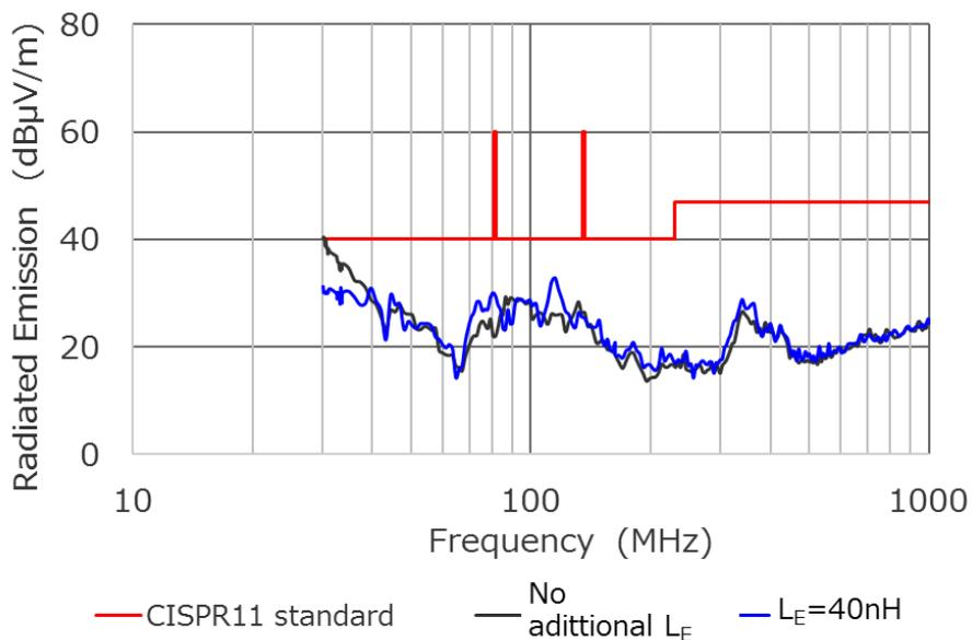
Figure. 3-3 Radiated Emission by adding  $L_E$  in IH rice cooker (actual measurement)
