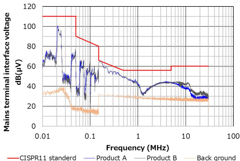
a) Example of conduction noise (actual measurement)
