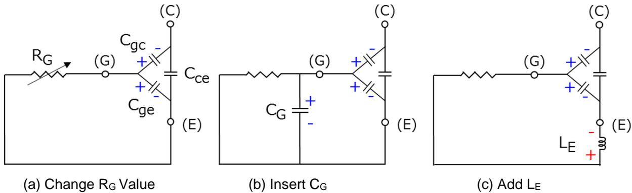
**Figure. 3-4 Simple model to study counter measures to suppress radiation noise and issues on switching characteristics.**
