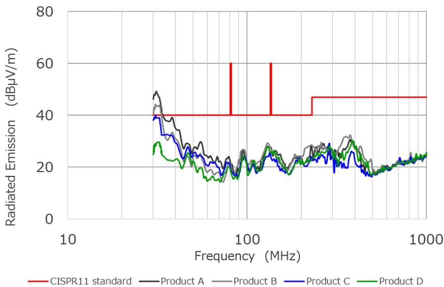
**Figure. 1-3 Differences in Radiated Emission in IH Rice Cooker by IGBT Products
