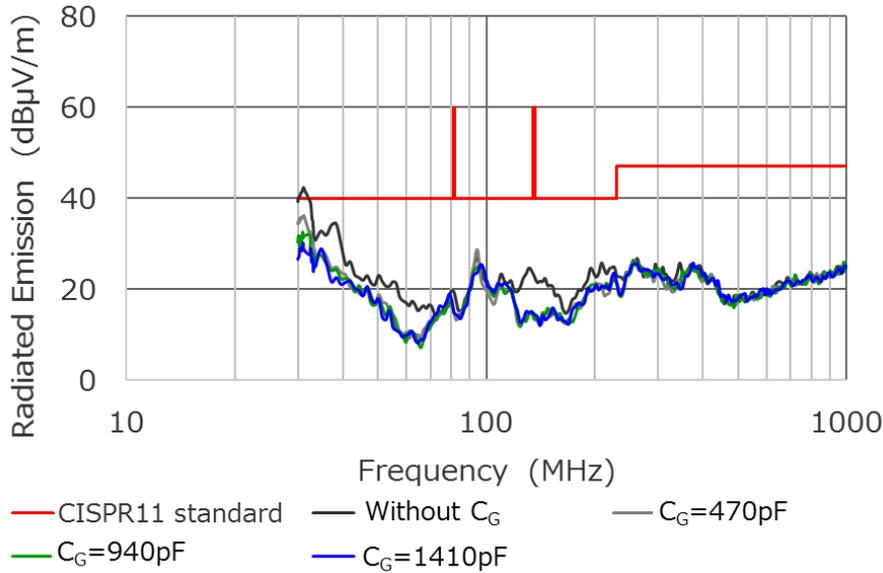
Figure. 3-2 Radiated Emission by inserting  $C_G$  in IH rice cooker (actual measurement)
