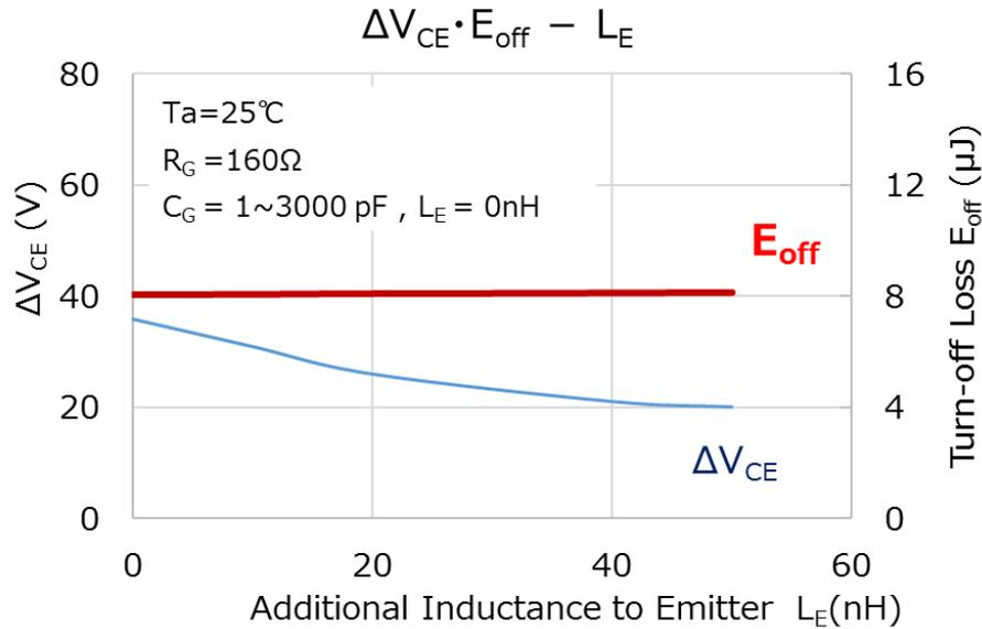
**Figure. 3-11  $L_E$  Effects on Turnoff Loss and “ $\Delta V_{CE}$ ” (Simulation)**
