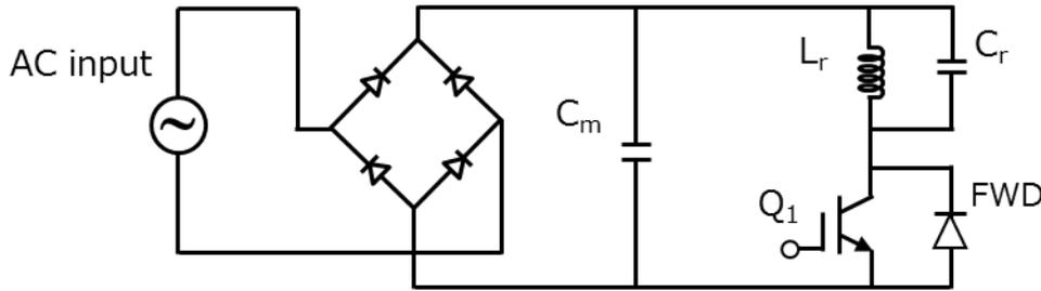
Figure. 2-1 Voltage Resonant Circuits Using IGBT
