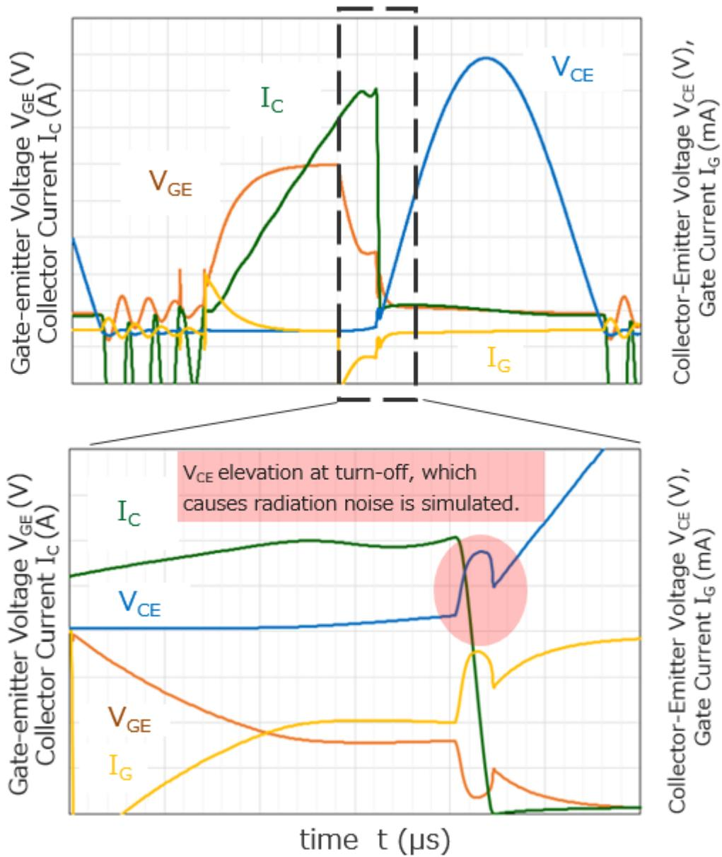
Figure. 3-8 Voltage Resonance Waveform for IH Rice Cooker (Simulation)
