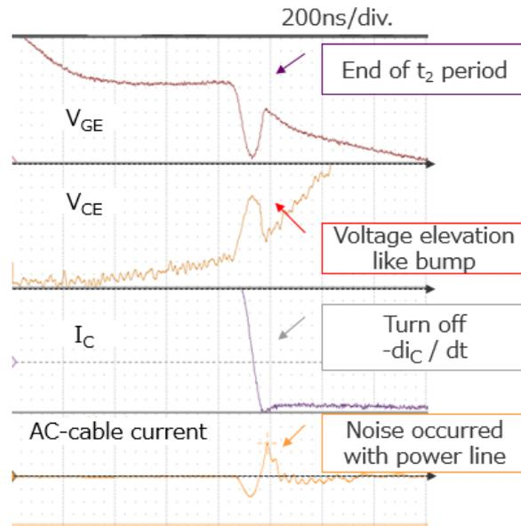
(b) Example of turn-off waveform (actual measurement)
