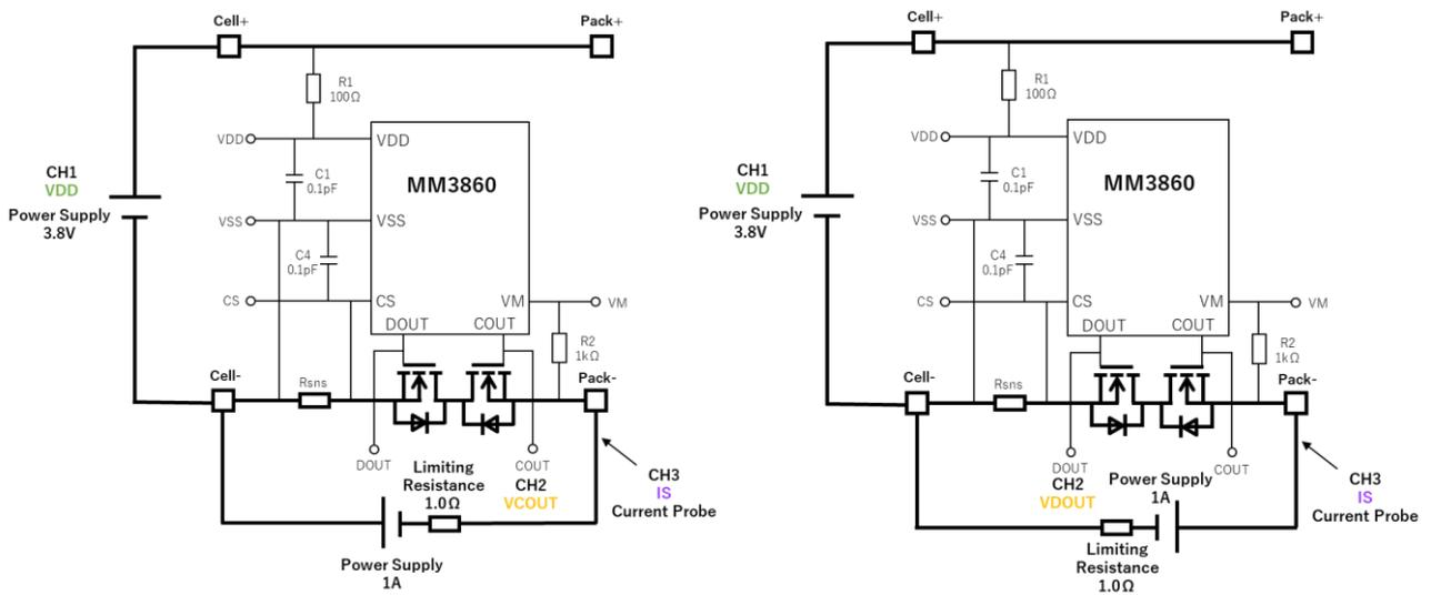
**Figure 5.1 Overcharge Voltage Measurement Circuit (Left) and Overdischarge Voltage Measurement Circuit (Right)**
