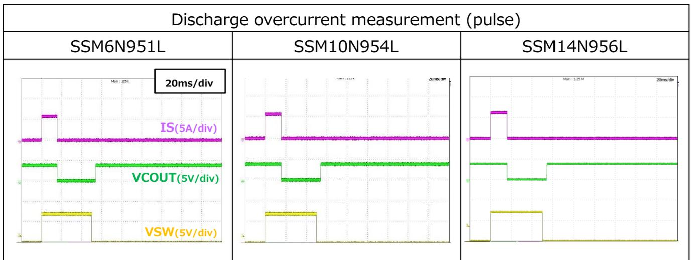
**Figure 5.8 Discharge Overcurrent Pulse Measurement Results**
