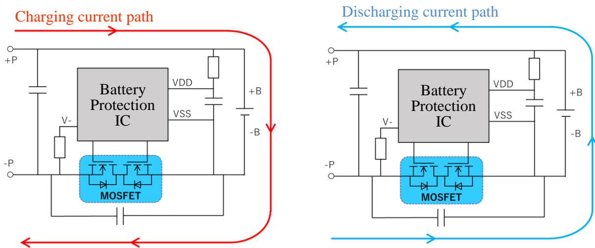
**Figure 3.1 Current Direction during Charging and Discharging**
