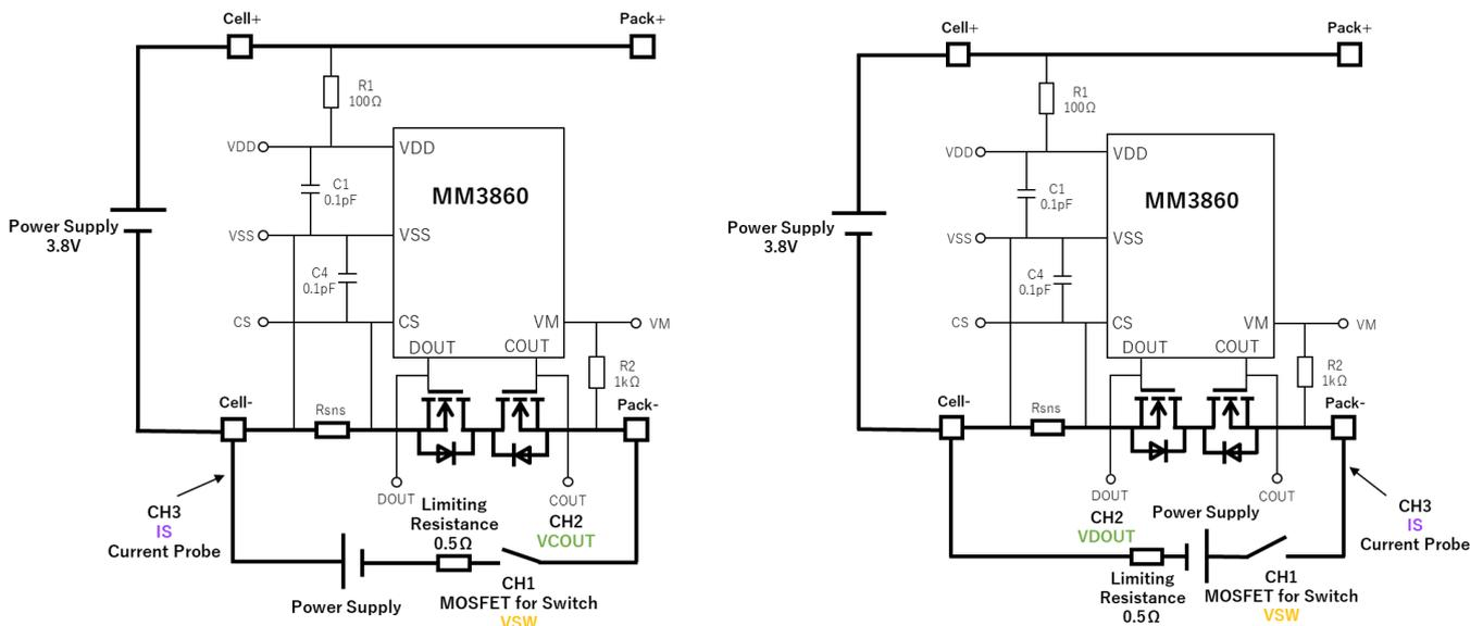
**Figure 5.4 Charge Overcurrent Measurement Circuit (Left) and Discharge Overcurrent Measurement Circuit (Right)**
