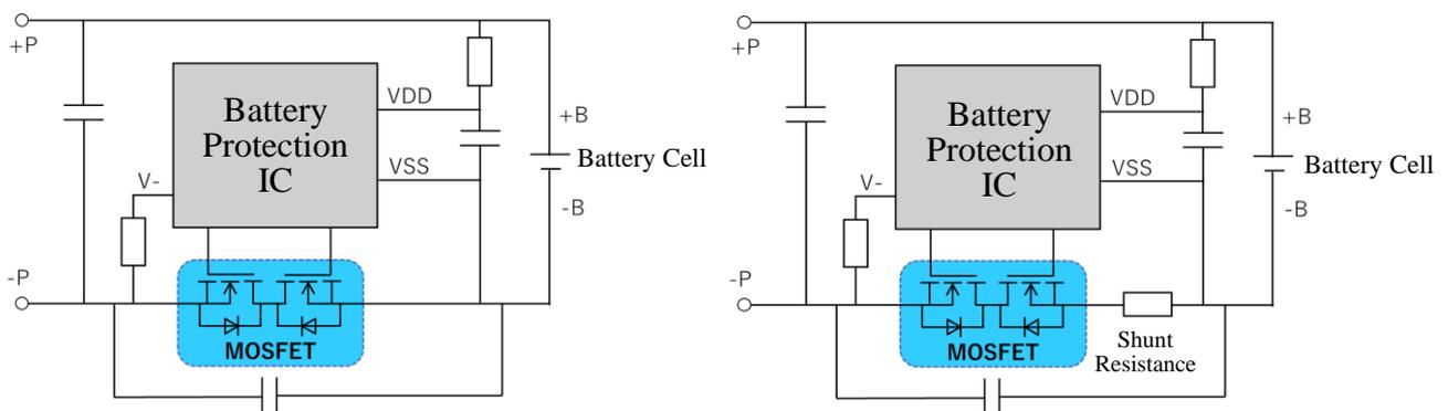
**Figure 2.2 Example of Typical Protection Circuit Block Diagram**
