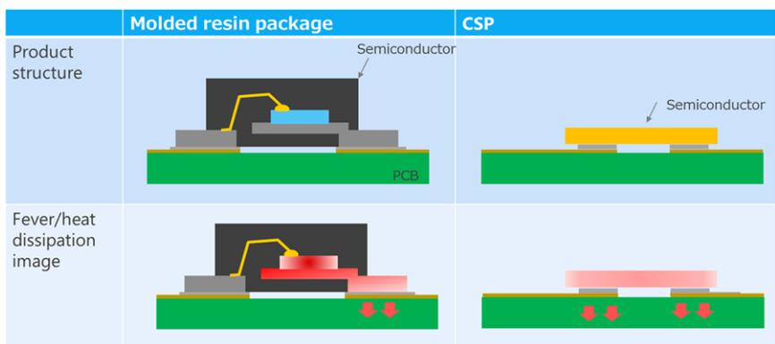
**Figure 4.1 Comparison Image of Molded Resin Package and CSP Package**
