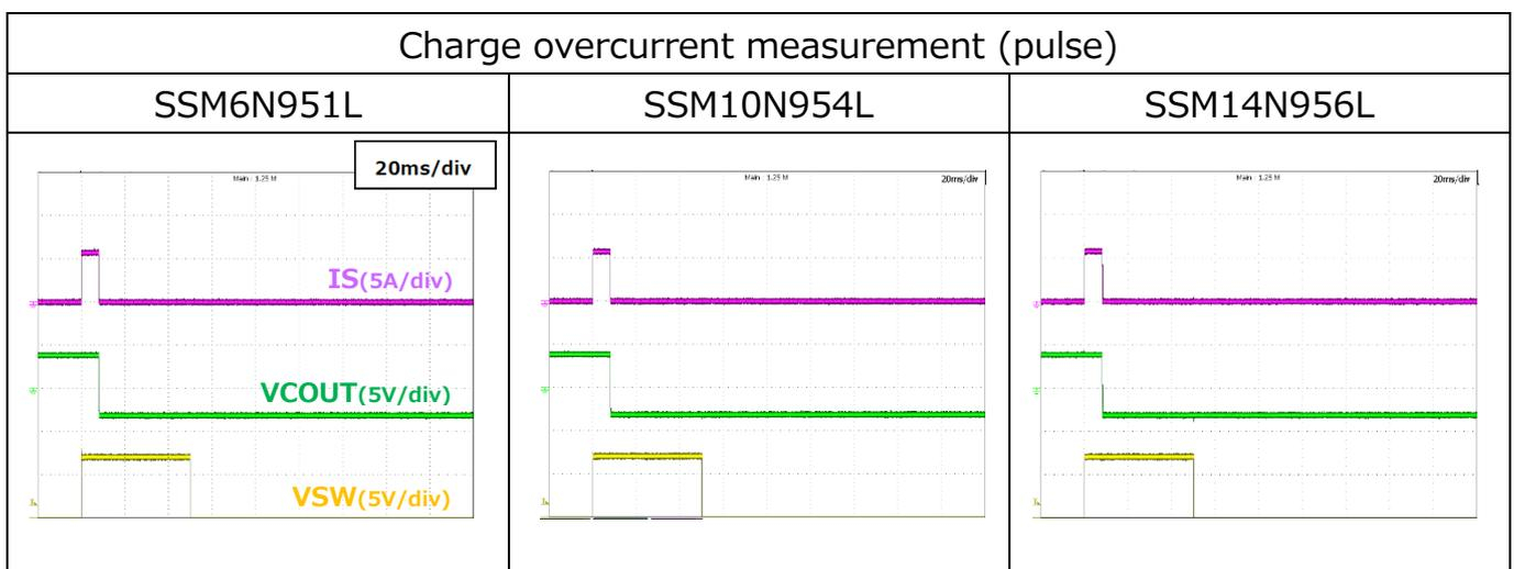
**Figure 5.6 Charge Overcurrent Pulse Measurement Results**
