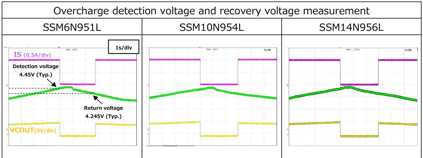
**Figure 5.2 Overcharge Voltage Measurement Results**
