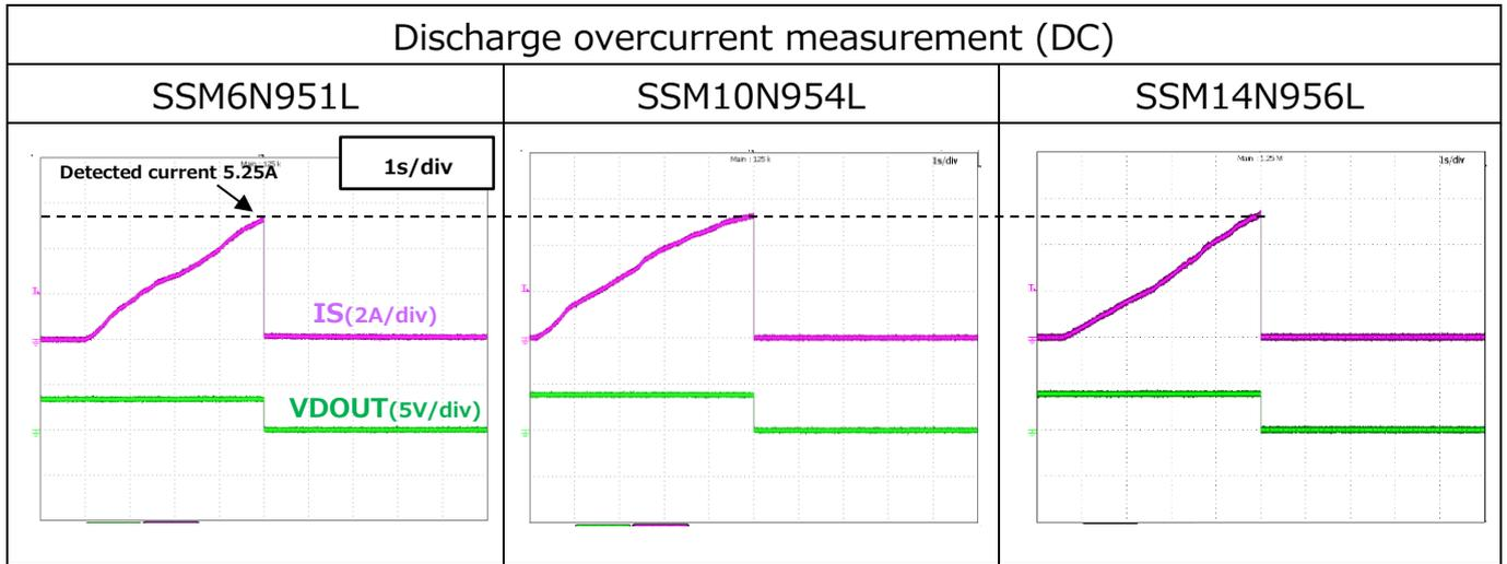
**Figure 5.7 Discharge Overcurrent DC Measurement Results**
