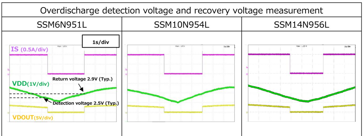
**Figure 5.3 Overdischarge Voltage Measurement Results**
