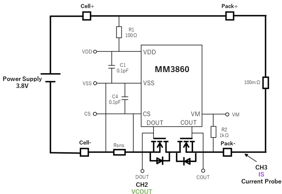
**Figure 5.9 Circuit Diagram for Short-Circuit Measurement**
