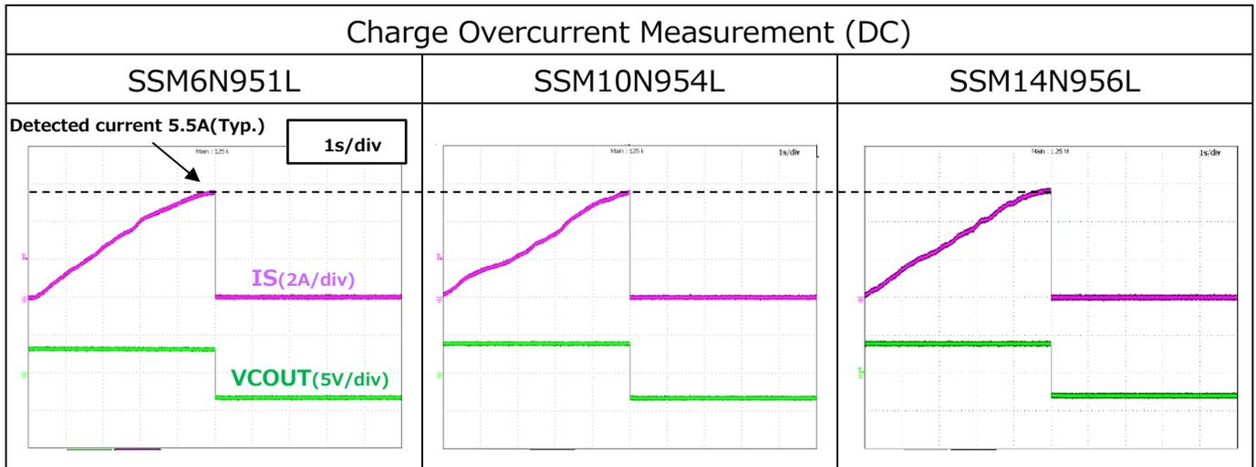
**Figure 5.5 Charging Overcurrent DC Measurement Results**
